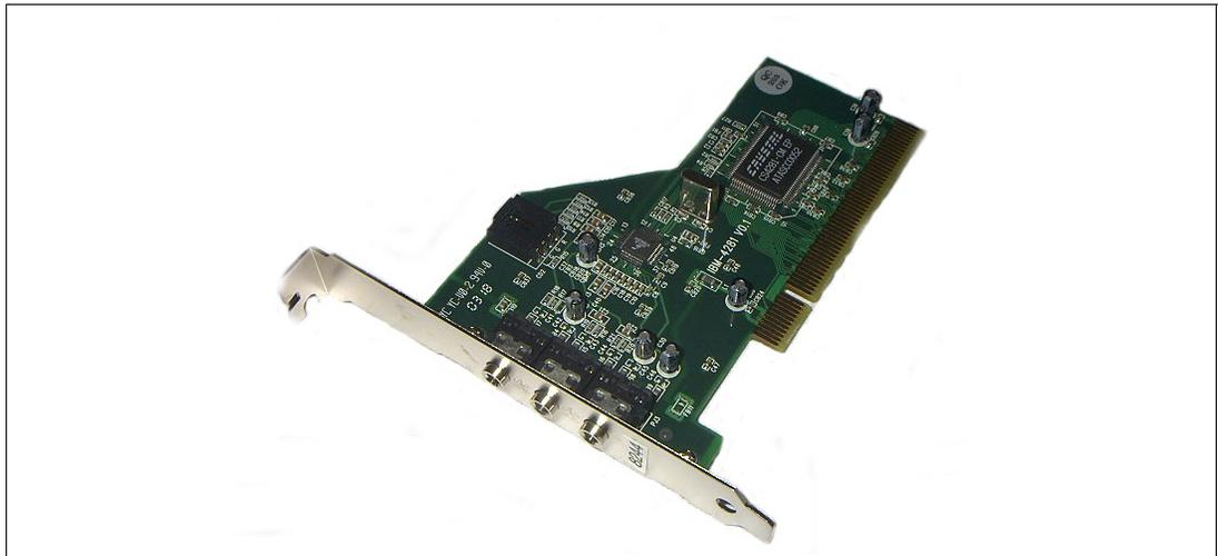
Figure 2-9 PCI audio adapter
