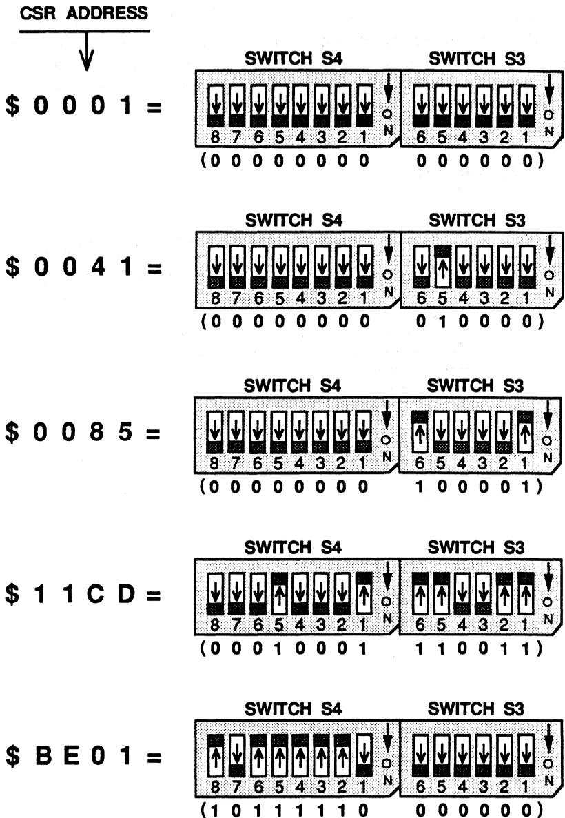
Figure 2-3. CSR Address Mapping Examples
