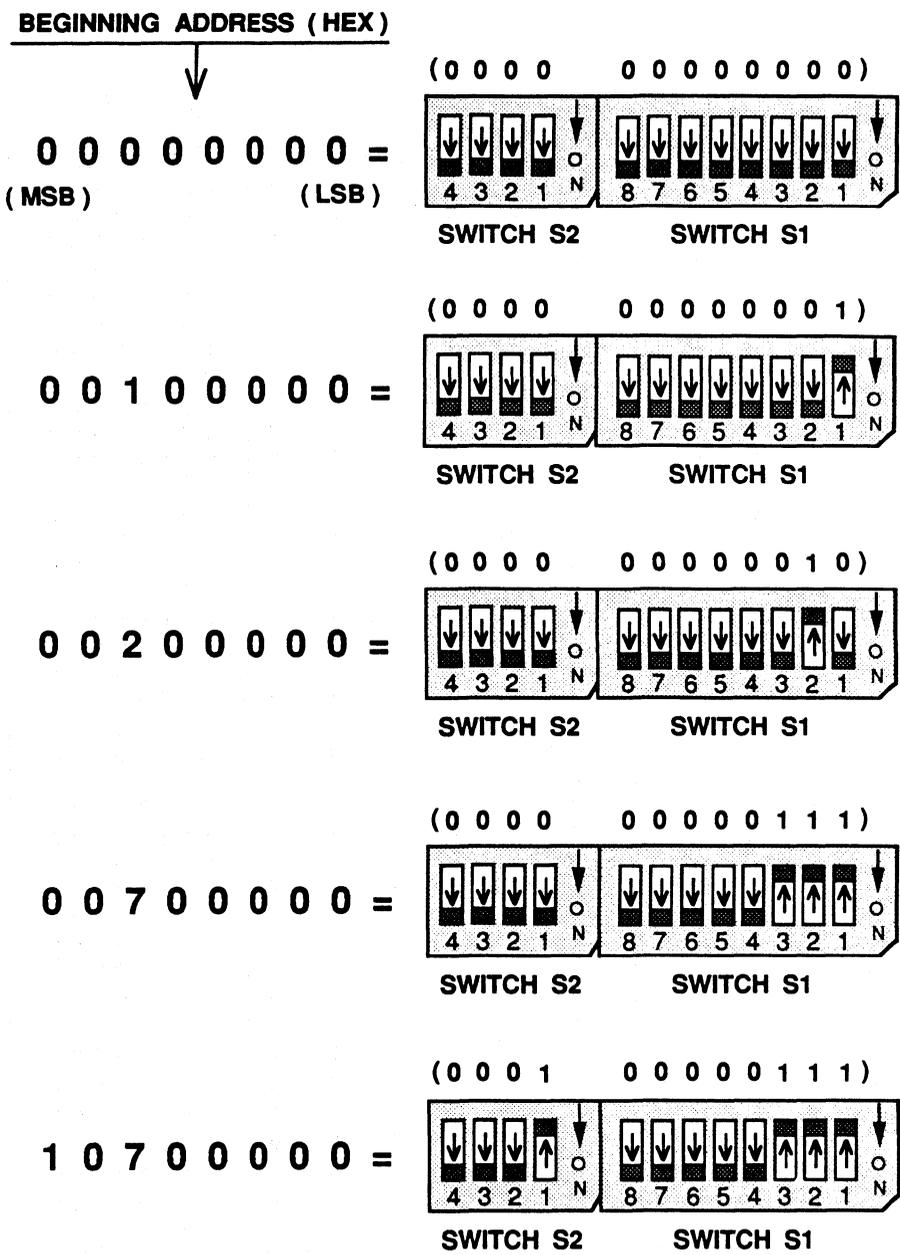
Figure 2-2. VMEbus Address Mapping Examples
