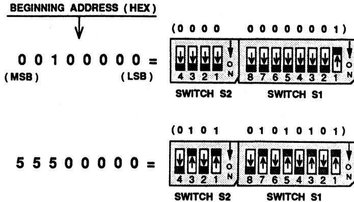
The switches should be ON for 0 and OFF for 1. Thus, a starting address of 00100000 would have the following switch positions: S1-2 through S1-8 ON; S2-1 through S2-4 ON; and S1-1 OFF. A starting address of 55500000 would have switch positions S1-1, S1-3, S1-5, S1-7, S2-1, and S2-3 OFF, and the rest ON.
