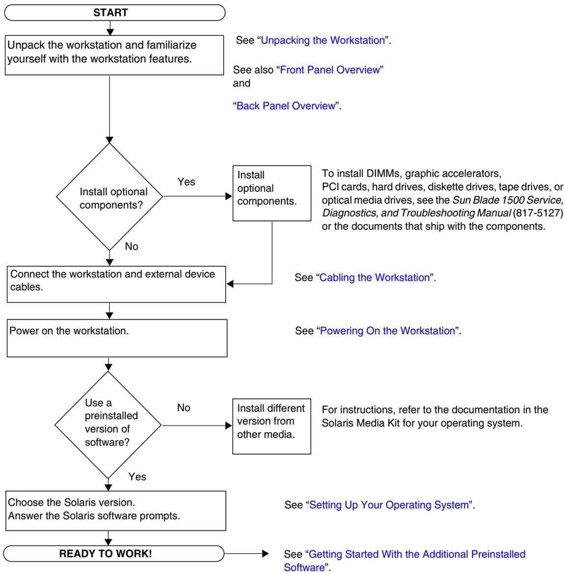
**FIGURE 1-1** Process for Installing the Sun Blade 1500 Workstation
