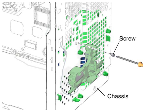
**FIGURE 13-41** Installing the Screw for the Front Fan Bracket
