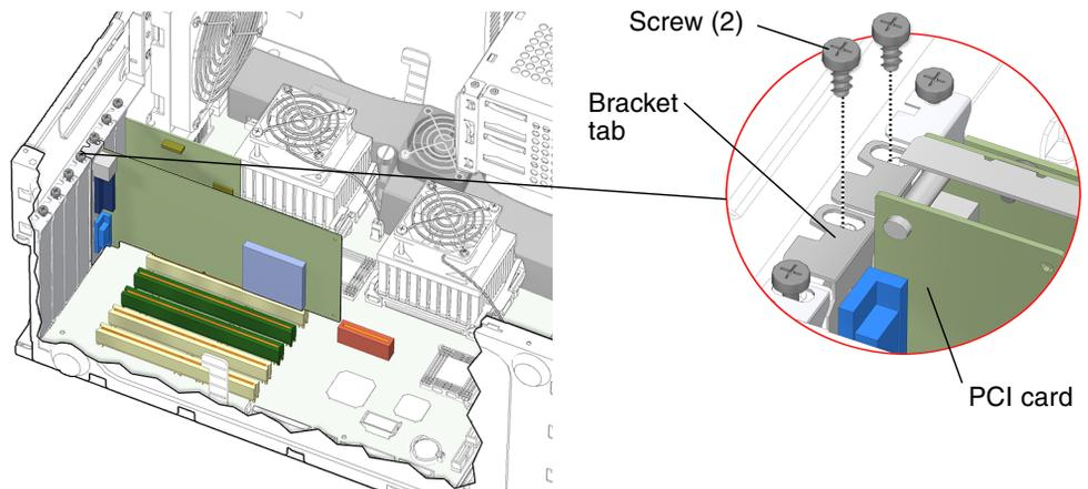
**FIGURE 11-38** Removing the PCI Card Bracket Tab Screw
