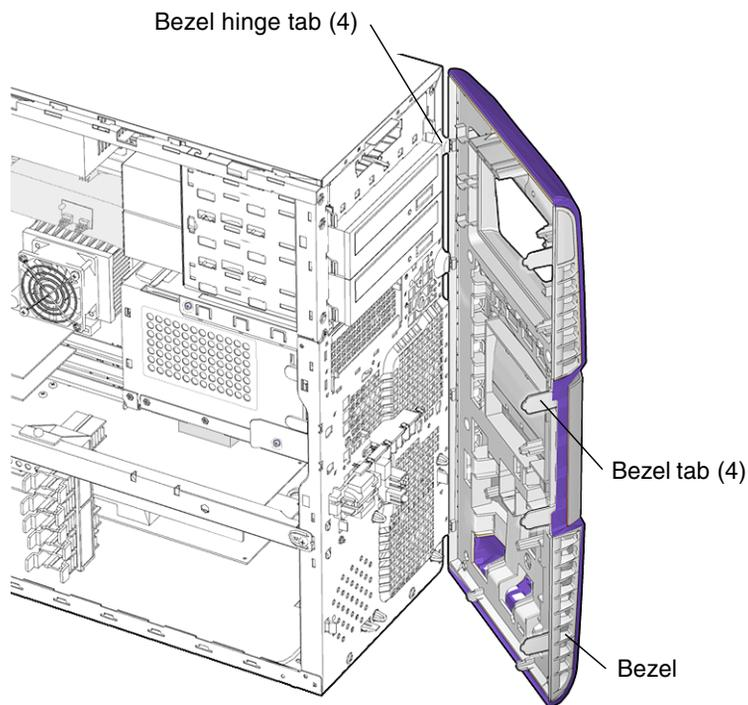
FIGURE 10-12 Removing the Bezel
