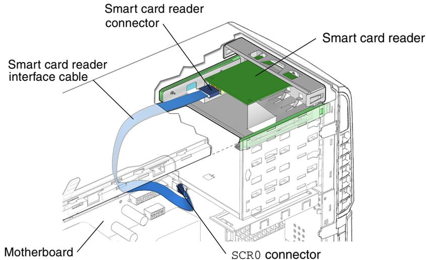
**FIGURE 14-3** Removing the Smart Card Reader Cable
