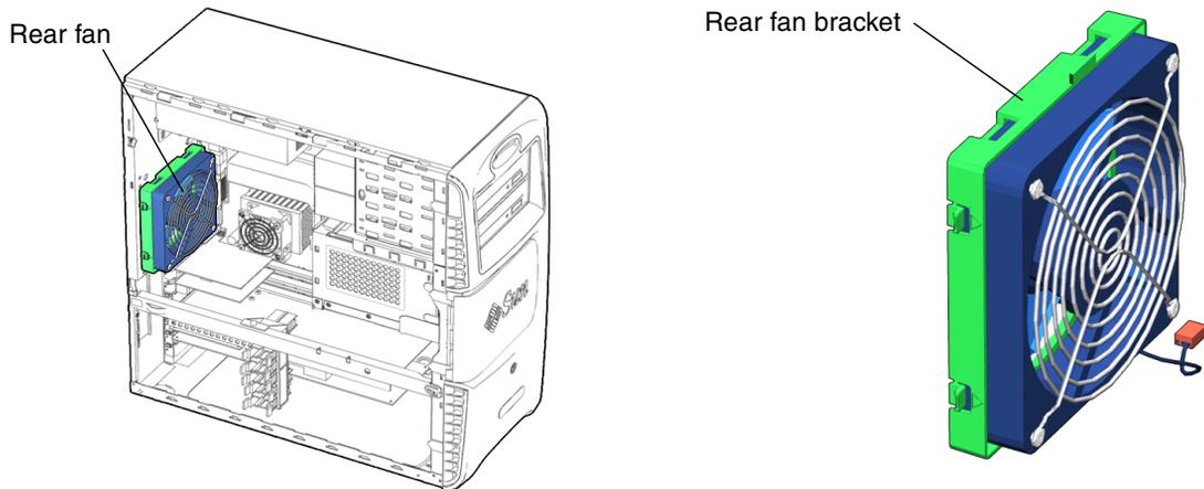
**FIGURE 13-16** Rear Fan Location and Identification
