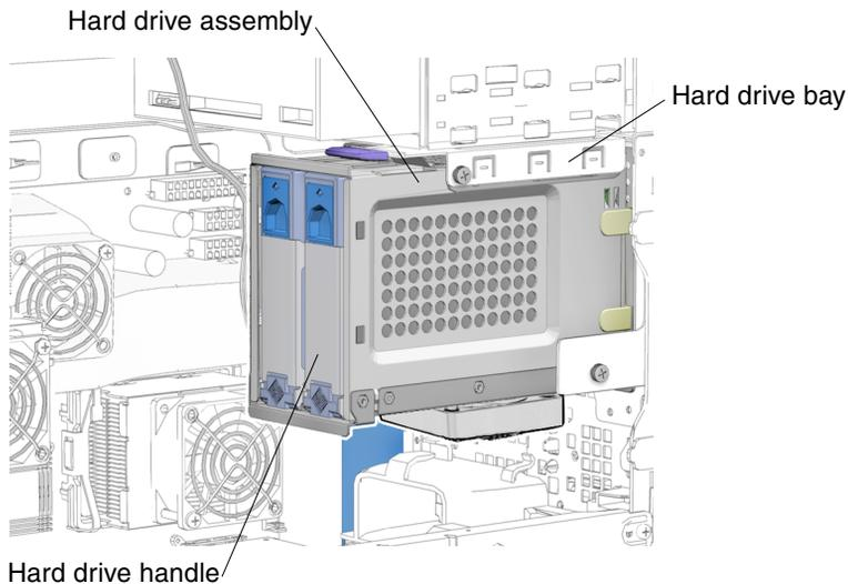
**FIGURE 12-6** Installing the Hard Drive in the Hard Drive Assembly
