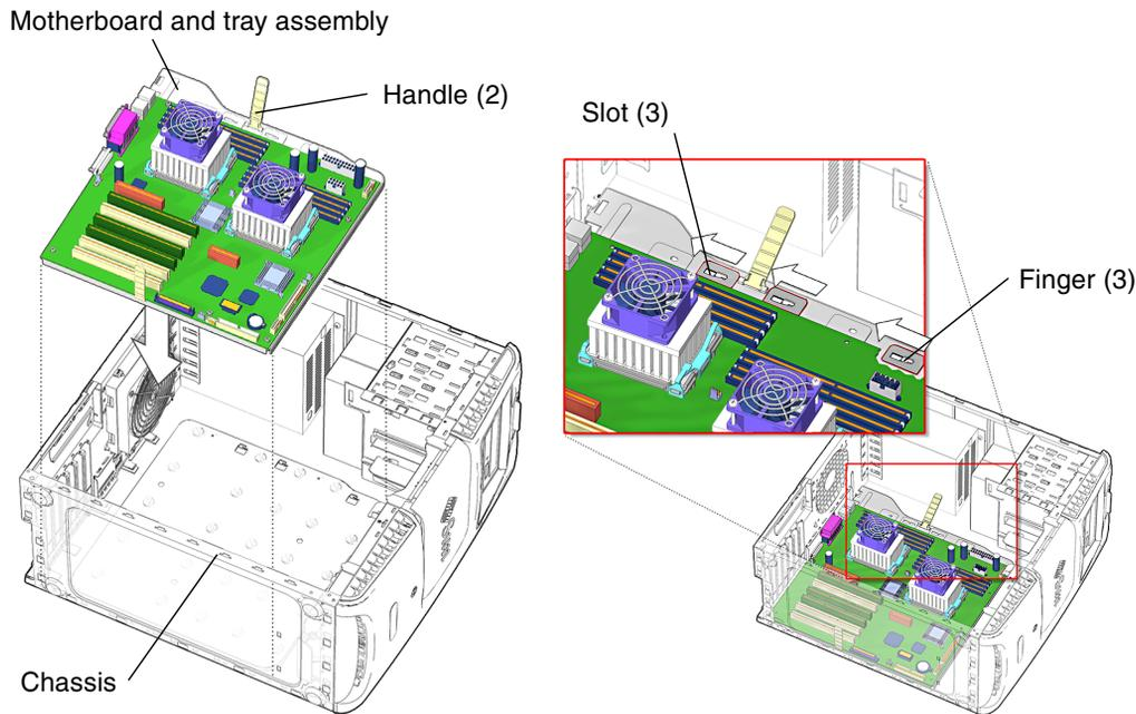
**FIGURE 11-50** Inserting the Motherboard and Tray Assembly Into the Chassis
