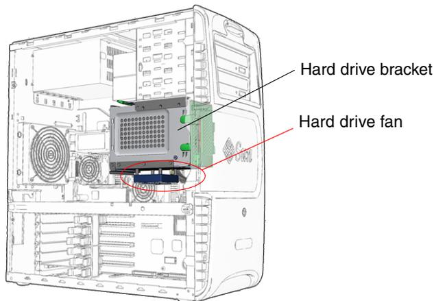
**FIGURE 13-22** Hard Drive Fan Location and Identification
