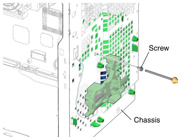
**FIGURE 13-37** Installing the Screw for the Front Fan Bracket
