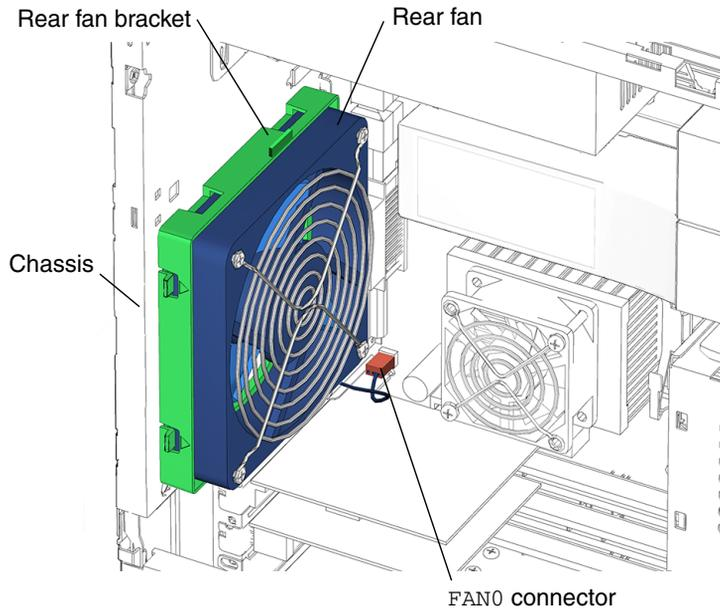
**FIGURE 13-21** Connecting the FAN0 Connector
