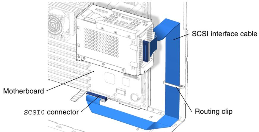
**FIGURE 14-11** Disconnecting the SCSI Interface Cable From the Motherboard
