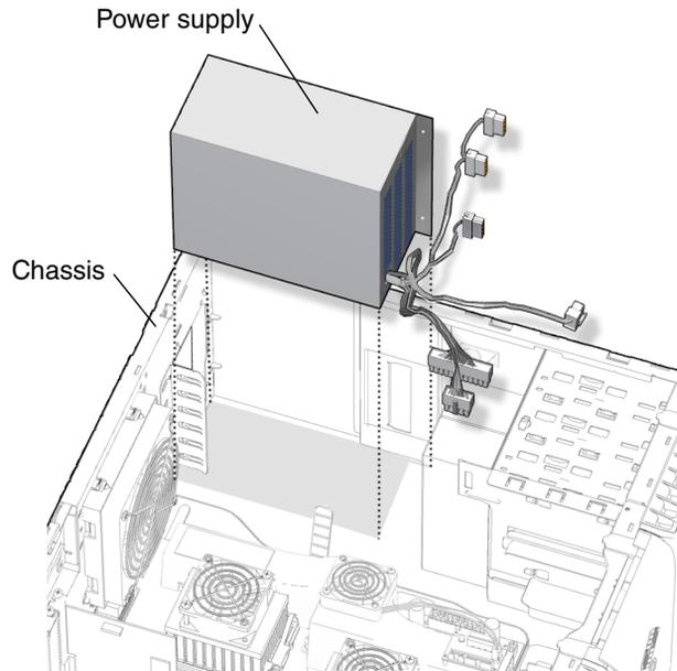
**FIGURE 13-6** Removing the Power Supply from the Chassis
