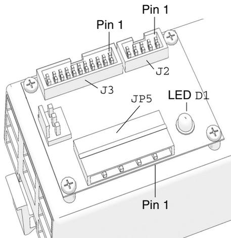
**FIGURE B-19** Interposer Board Connectors and Pin Configuration
