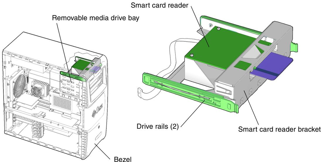
**FIGURE 12-15** Smart Card Reader Location and Identification
