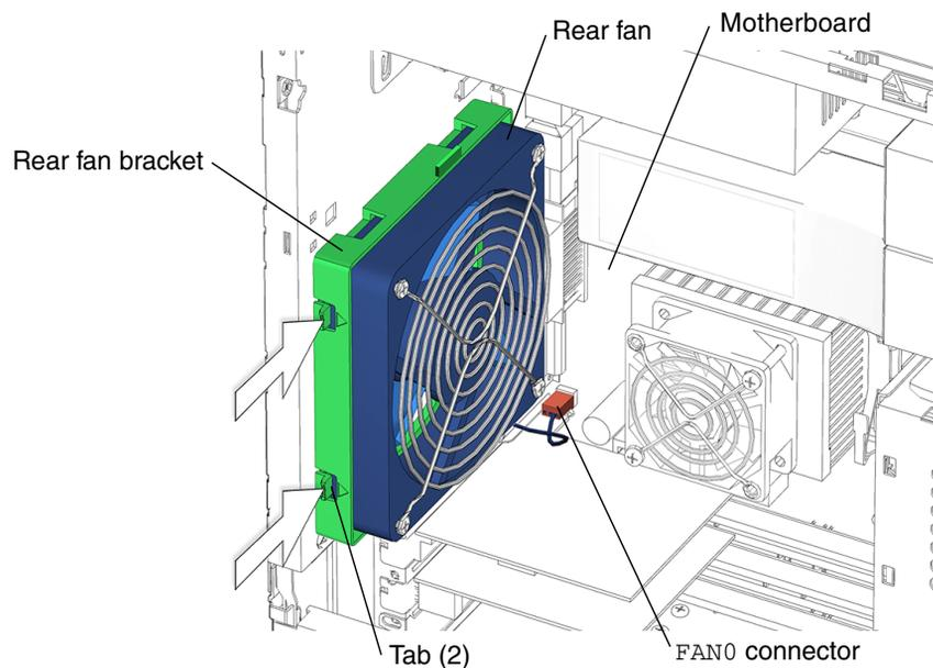
**FIGURE 13-17** Releasing the Rear Fan Assembly
