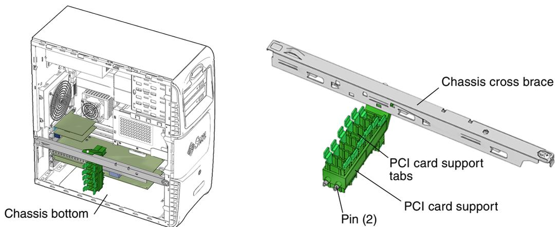
**FIGURE 13-39** PCI Card Support Location and Identification
