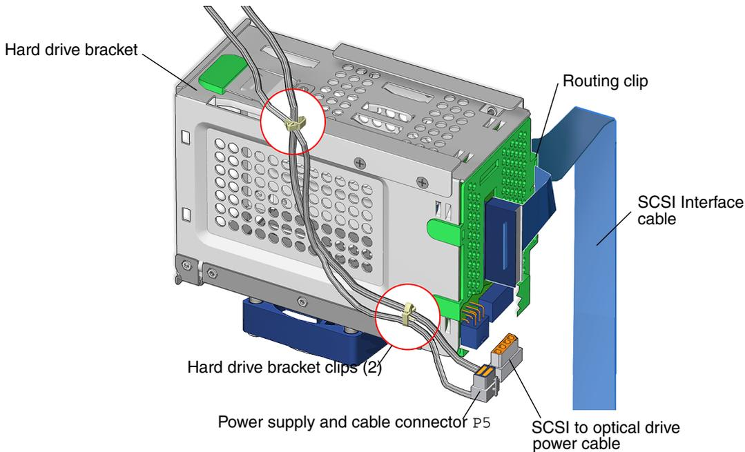
**FIGURE 10-16** Disconnecting the Hard Drive Bracket Cables
