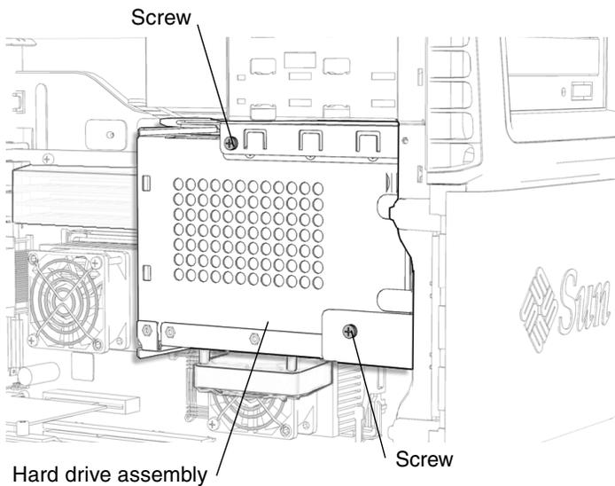
**FIGURE 15-3** Installing the Hard Drive Assembly Screws
