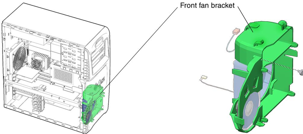
**FIGURE 13-33** Front Fan Bracket Location and Identification
