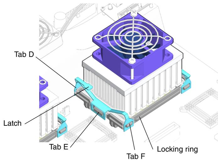
**FIGURE 11-29** Installing the Clip Over Tab E
