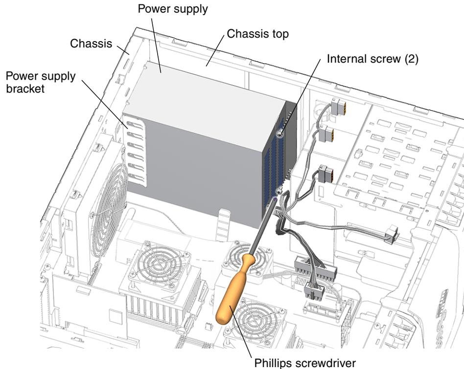
**FIGURE 13-7** Aligning the Power Supply to the Chassis
