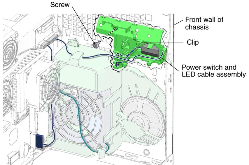
**FIGURE 13-34** Loosening the Power Switch and LED Cable Assembly From the Chassis
