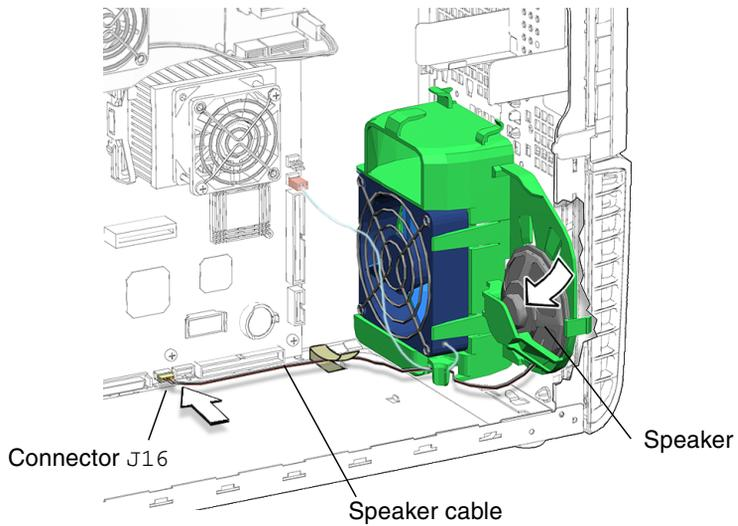
**FIGURE 13-32** Aligning and Installing the Speaker and Cable
