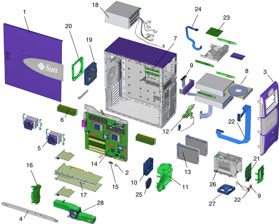
FIGURE 10-17 Workstation Components
