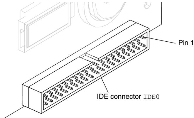
**FIGURE B-17** IDE Connector IDE0 Pin Configuration
