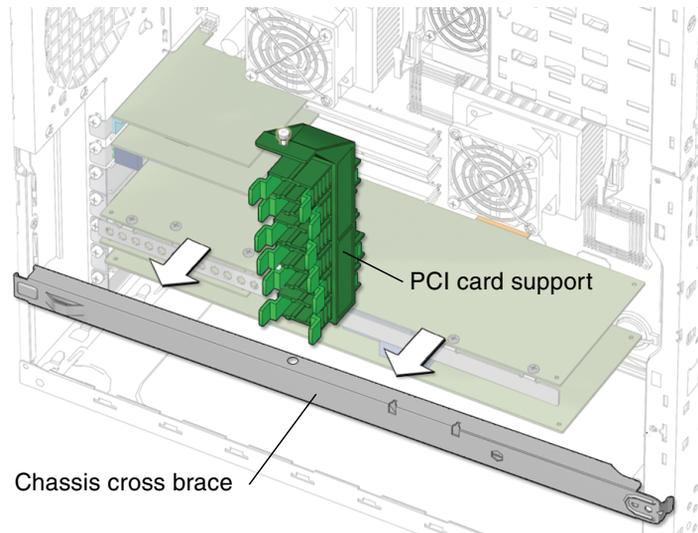
**FIGURE 13-42** Removing Chassis Cross Brace and PCI Card Support
