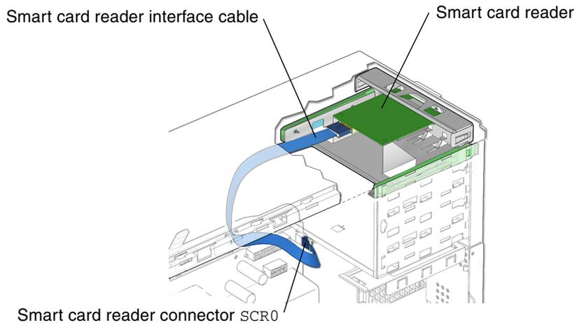
**FIGURE 12-19** Connecting the Smart Card Reader Cable
