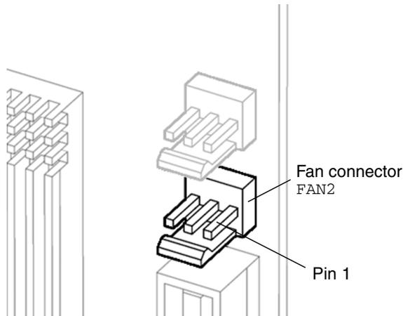
**FIGURE B-15** Fan Connector FAN2 Pin Configuration
