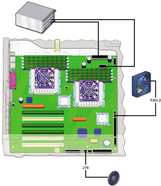
**FIGURE 11-53** Installing Motherboard Power Cables
