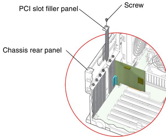
**FIGURE 11-40** Installing a PCI Slot Filler Panel
