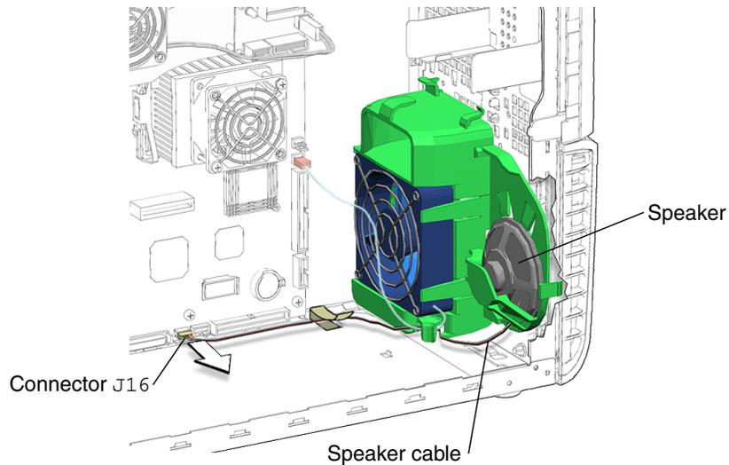
**FIGURE 13-30** Disconnecting the Speaker Cable
