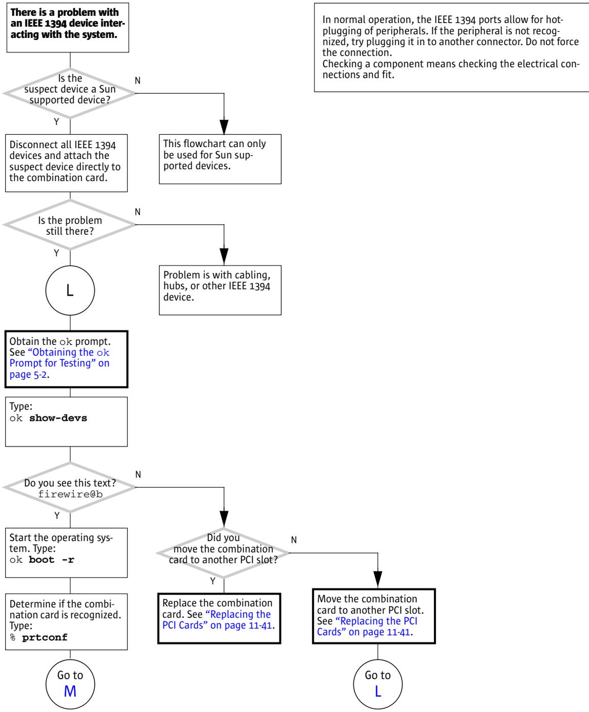
In normal operation, the IEEE 1394 ports allow for hot-plugging of peripherals. If the peripheral is not recognized, try plugging it in to another connector. Do not force the connection. Checking a component means checking the electrical connections and fit.
