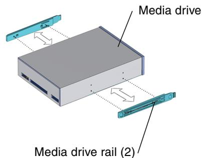
**FIGURE 13-49** Installing Drive Rails on a Media Drive
