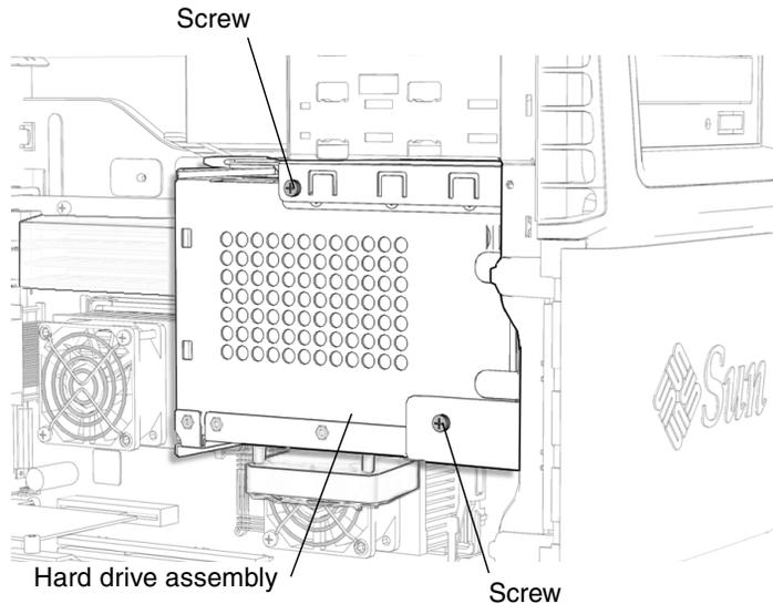
**FIGURE 14-9** Installing the Hard Drive Assembly Screws
