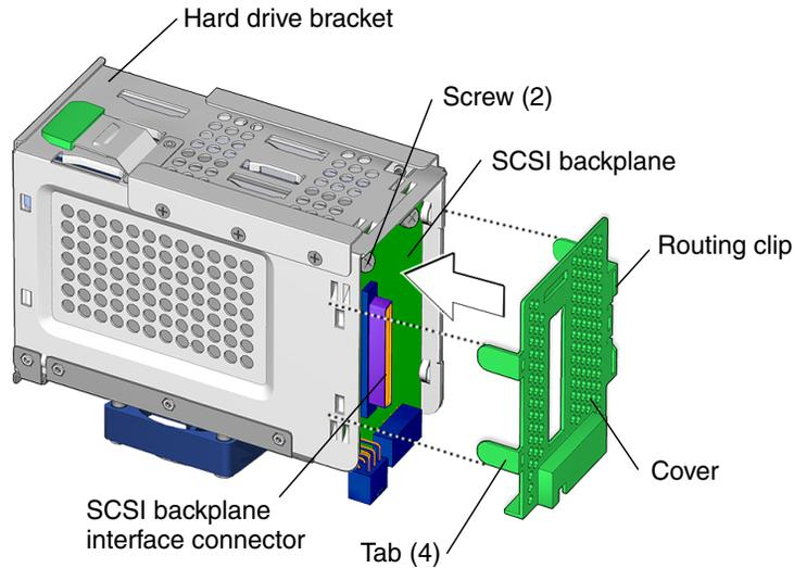
**FIGURE 13-28** Installing the SCSI Backplane Cover
