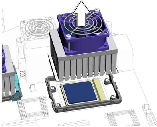
**FIGURE 11-24** Removing the CPU Fan and Heat Sink Assembly
