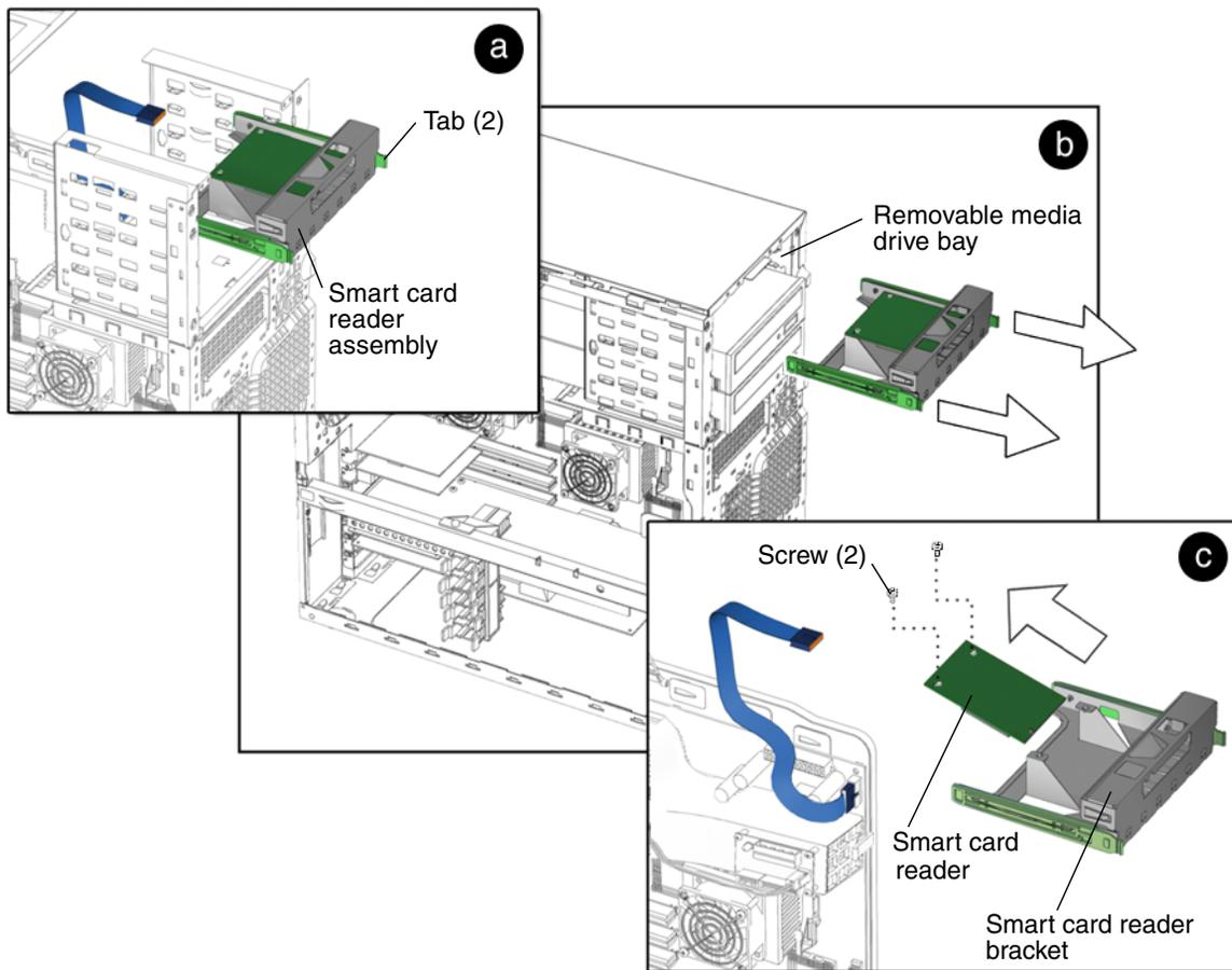
**FIGURE 12-17** Removing the Smart Card Reader Assembly
