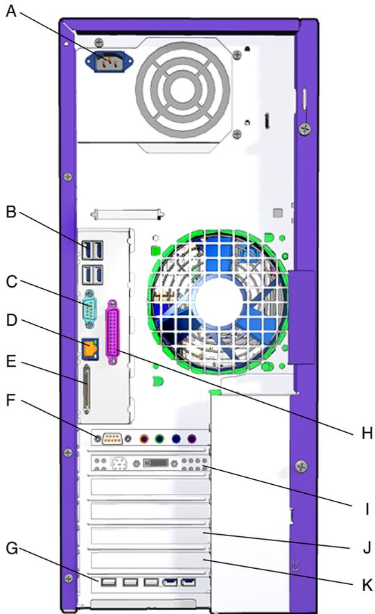
**FIGURE 2-3** Rear Panel Overview, Sun Blade 2500 Workstation
