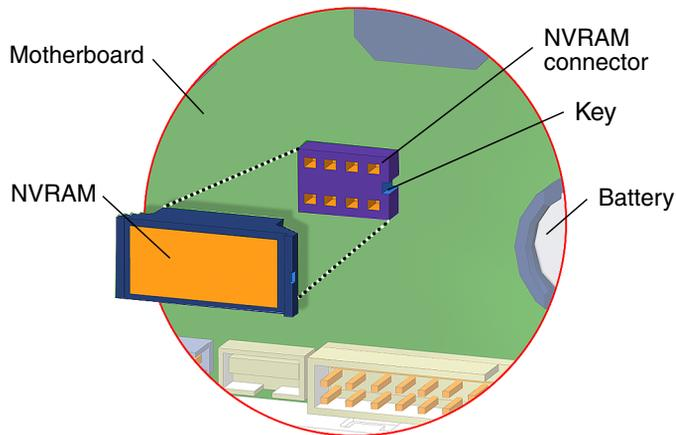
**FIGURE 11-35** Removing NVRAM
