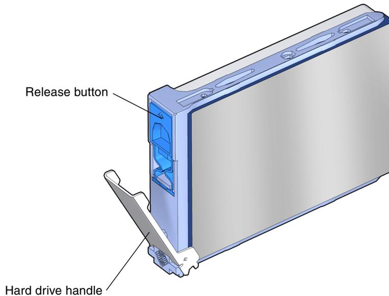
**FIGURE 12-4** Preparing the Hard Drive for Installation
