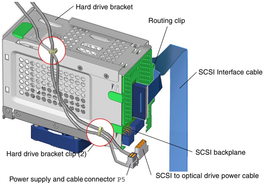
**FIGURE 15-1** Installing the Power and Signal Cables for the Hard Drive Assembly
