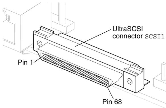
**FIGURE B-11** UltraSCSI Connector SCSI1 Pin Configuration
