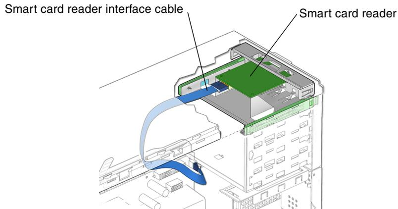
**FIGURE 12-16** Removing the Smart Card Reader Cable
