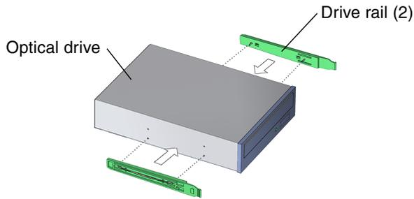
**FIGURE 12-12** Installing Drive Rails
