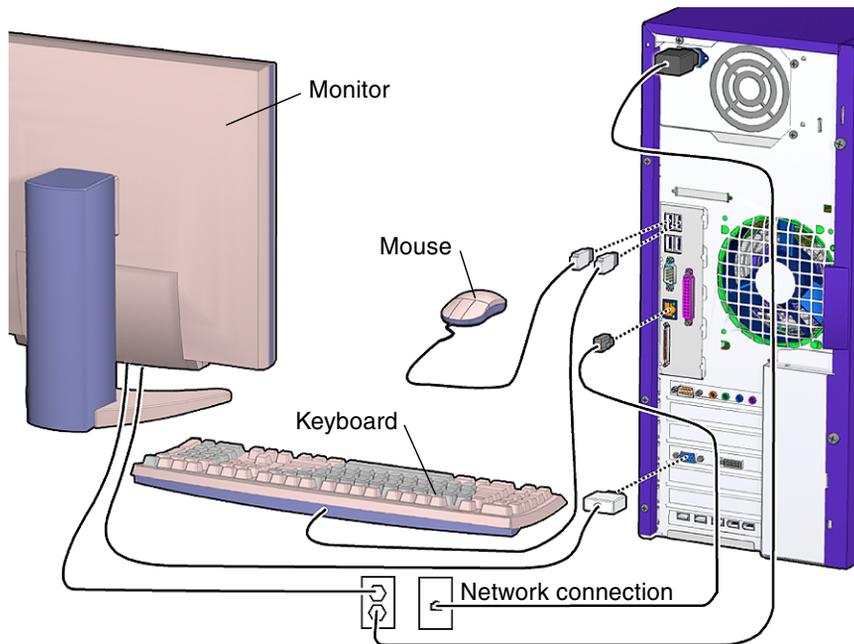
**FIGURE 15-7** Reconnecting the Keyboard, Mouse, Monitor, and Network
