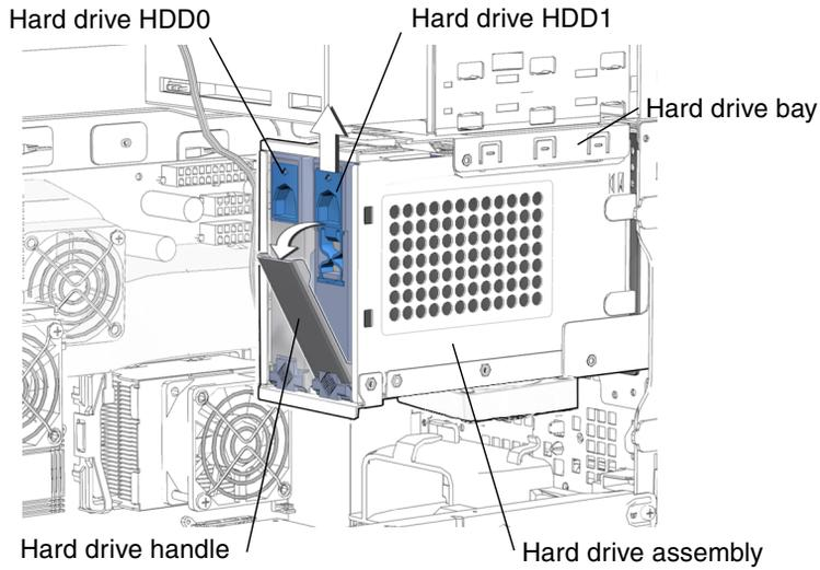
**FIGURE 12-2** Releasing the Hard Drive From the Hard Drive Assembly
