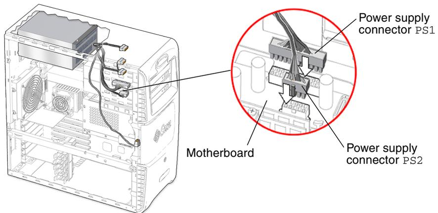
**FIGURE 13-9** Installing Power Supply Connectors PS1 and PS2 to the Motherboard
