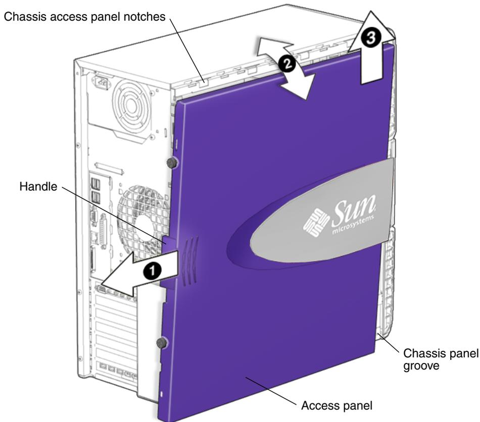
**FIGURE 10-8** Removing the Access Panel
