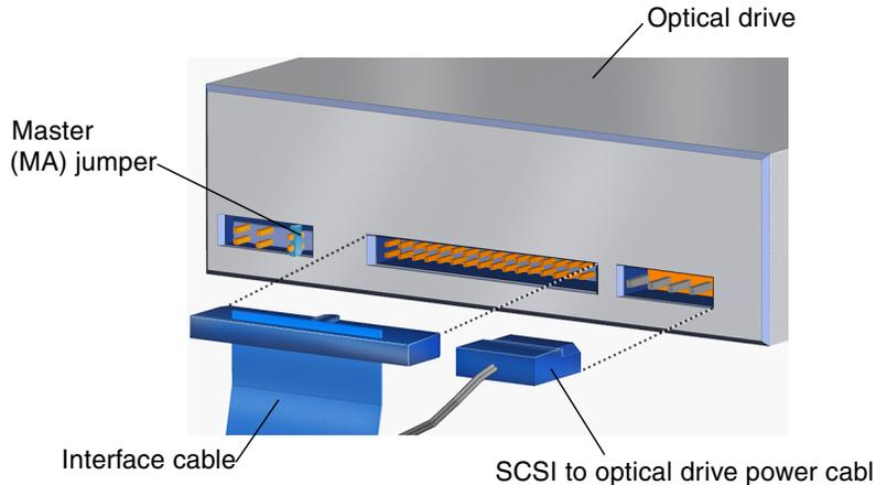
**FIGURE 12-13** Location of the Optical Drive Master Jumper
