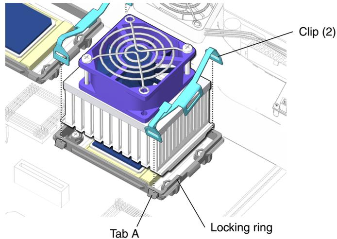
**FIGURE 11-25** Installing the Clip on Tab A
