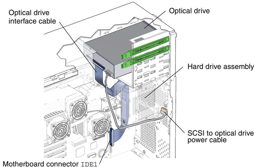
**FIGURE 14-4** Optical Drive Power and Interface Cables Location and Identification
