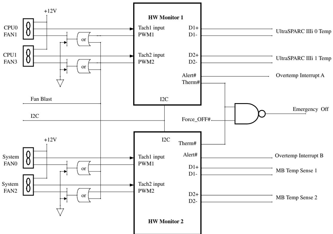
**FIGURE C-16** Fan Control and Temperature Sensing Block Diagram
