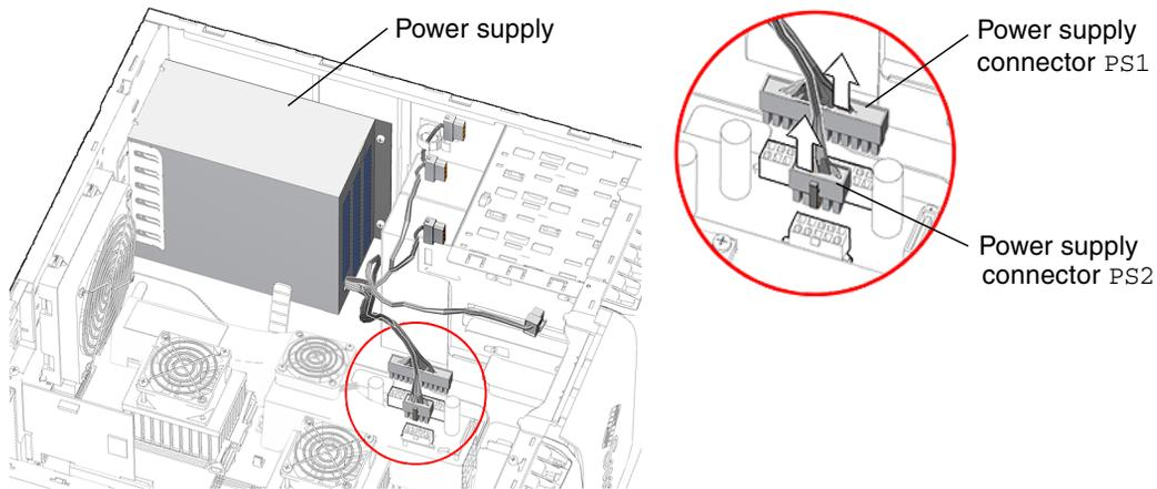
**FIGURE 13-3** Disconnecting the Power Supply Cables
