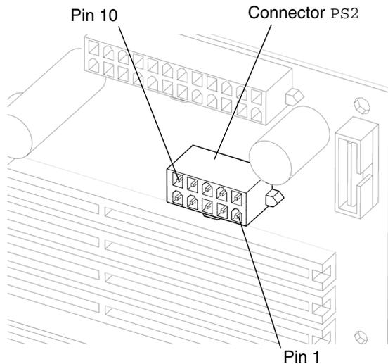
**FIGURE B-23** Power Supply Connector PS2 Pin Configuration
