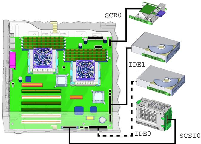
**FIGURE 11-47** Disconnecting Interface Cables
