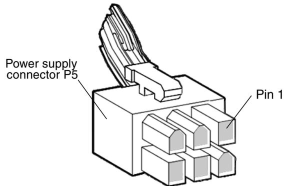
**FIGURE B-20** Power Supply Connector P5 Pin Configuration
