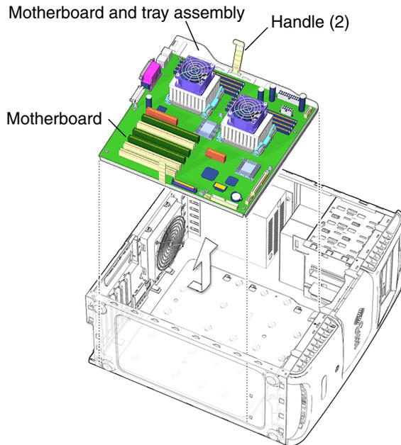
**FIGURE 11-49** Removing the Motherboard and Tray Assembly
