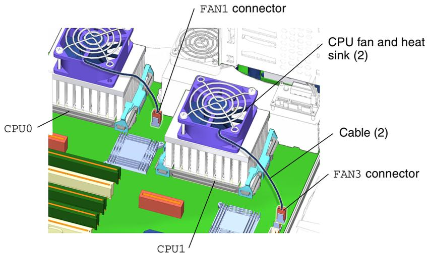
**FIGURE 11-30** Connecting CPU Fan and Heat Sink Assembly Connectors
