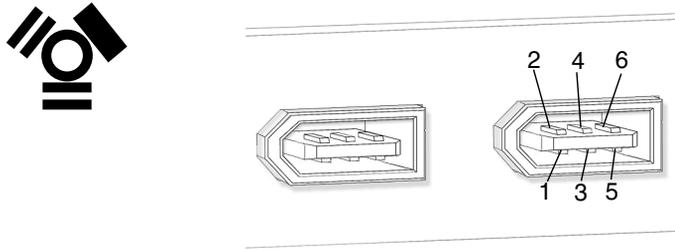
**FIGURE B-3** IEEE 1394a Connector Pin Configuration
