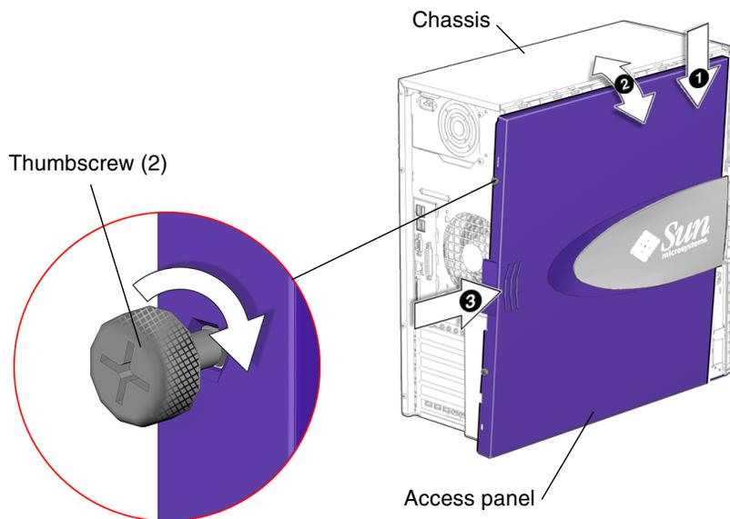
**FIGURE 15-6** Installing the Access Panel
