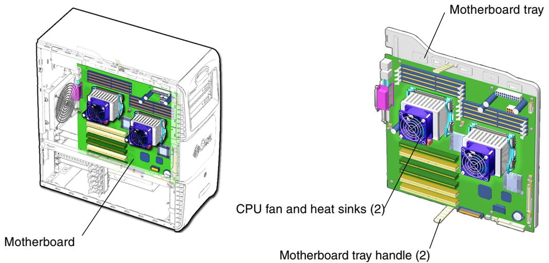
**FIGURE 11-43** Motherboard Location and Identification
