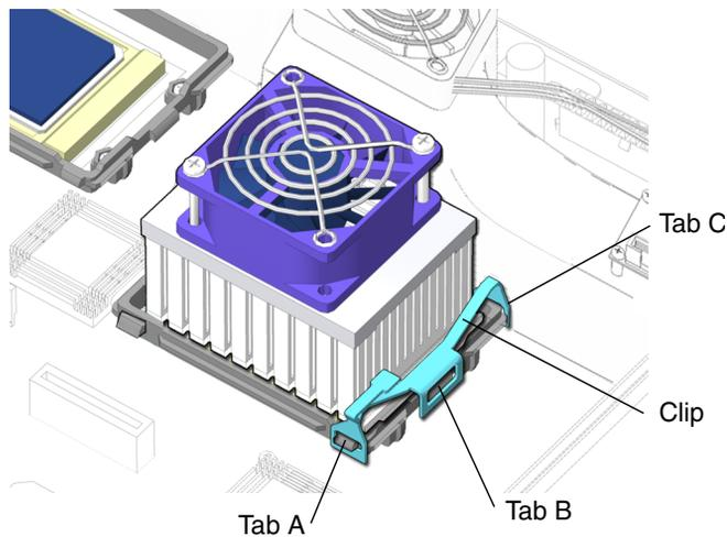
**FIGURE 11-27** Installing the Clip Into the Lock-Down Position
