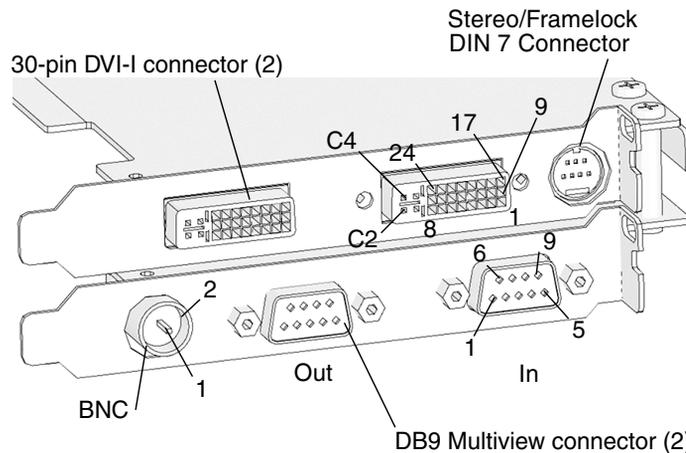
**FIGURE B-9** Sun XVR-1200 Graphics Accelerator Connectors Pin Configuration
