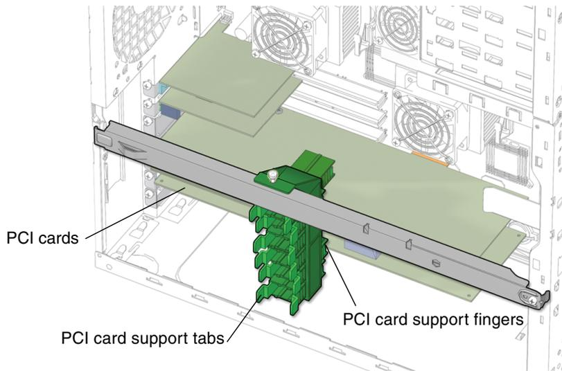
**FIGURE 13-45** Aligning the PCI Card Support Tabs
