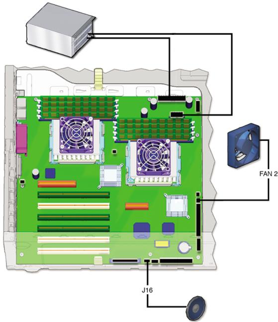
**FIGURE 11-46** Disconnecting Power Cables
