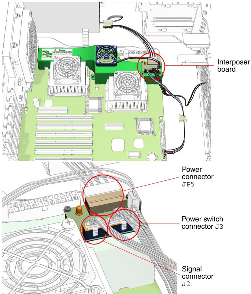
**FIGURE 11-12** Removing Cables From the Interposer Board
