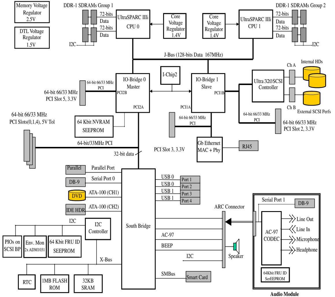
FIGURE C-1 Sun Blade 2500 System Block Diagram
