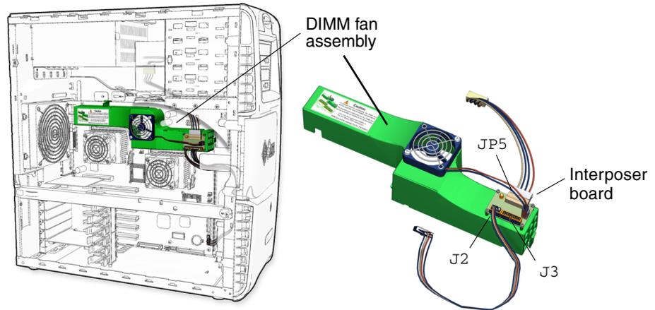
**FIGURE 11-9** DIMM Fan Assembly Location and Identification
