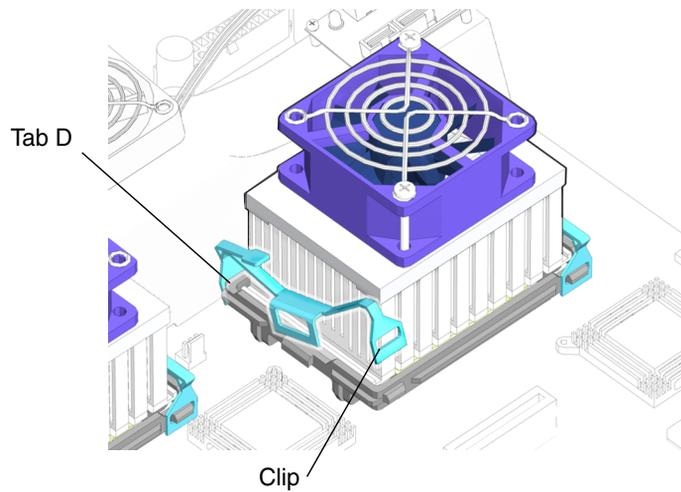
**FIGURE 11-28** Installing the Clip Over Tab D
