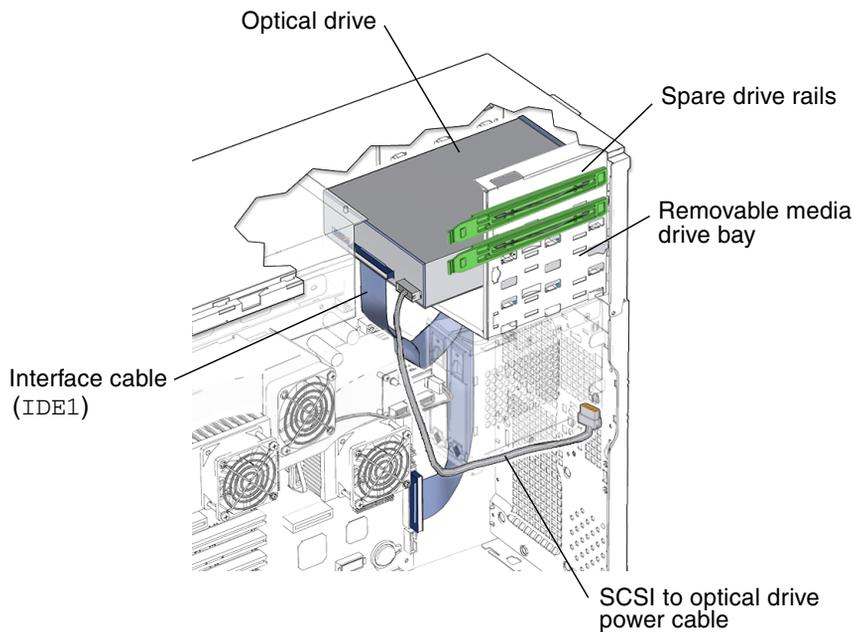
**FIGURE 12-8** Optical Drive Interface and Power Cables
