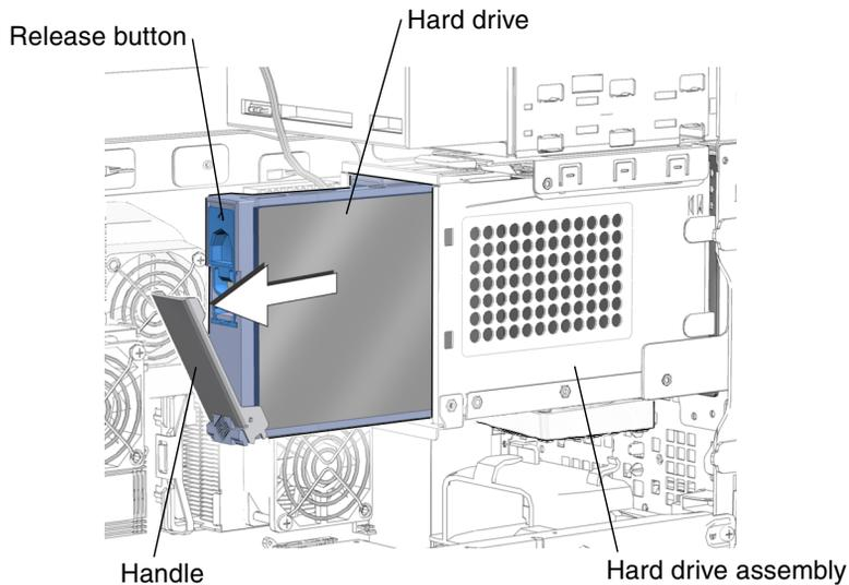
**FIGURE 12-3** Removing the Hard Drive From the Hard Drive Assembly
