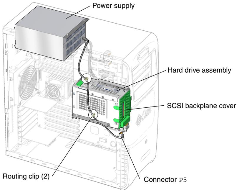
**FIGURE 13-2** Disconnecting Power Supply Cable Connector P5 From the Hard Drive Assembly
