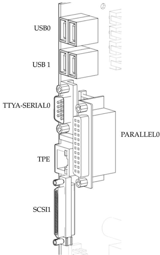
**FIGURE C-3** Motherboard Rear Connectors
