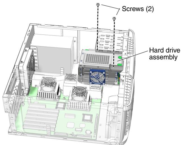
**FIGURE 11-10** Removing the Hard Drive Assembly Screws
