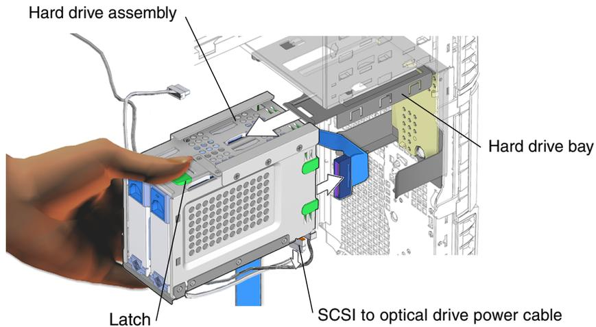
**FIGURE 14-6** Removing the Hard Drive Bracket Assembly
