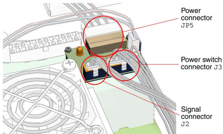
**FIGURE 11-15** Connecting Cables to the Interposer Board
