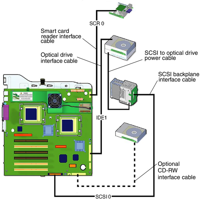
**FIGURE 14-1** Sun Blade 2500 Interface and Power Cables
