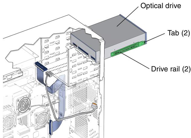
**FIGURE 12-9** Removing the Optical Drive and Drive Rails
