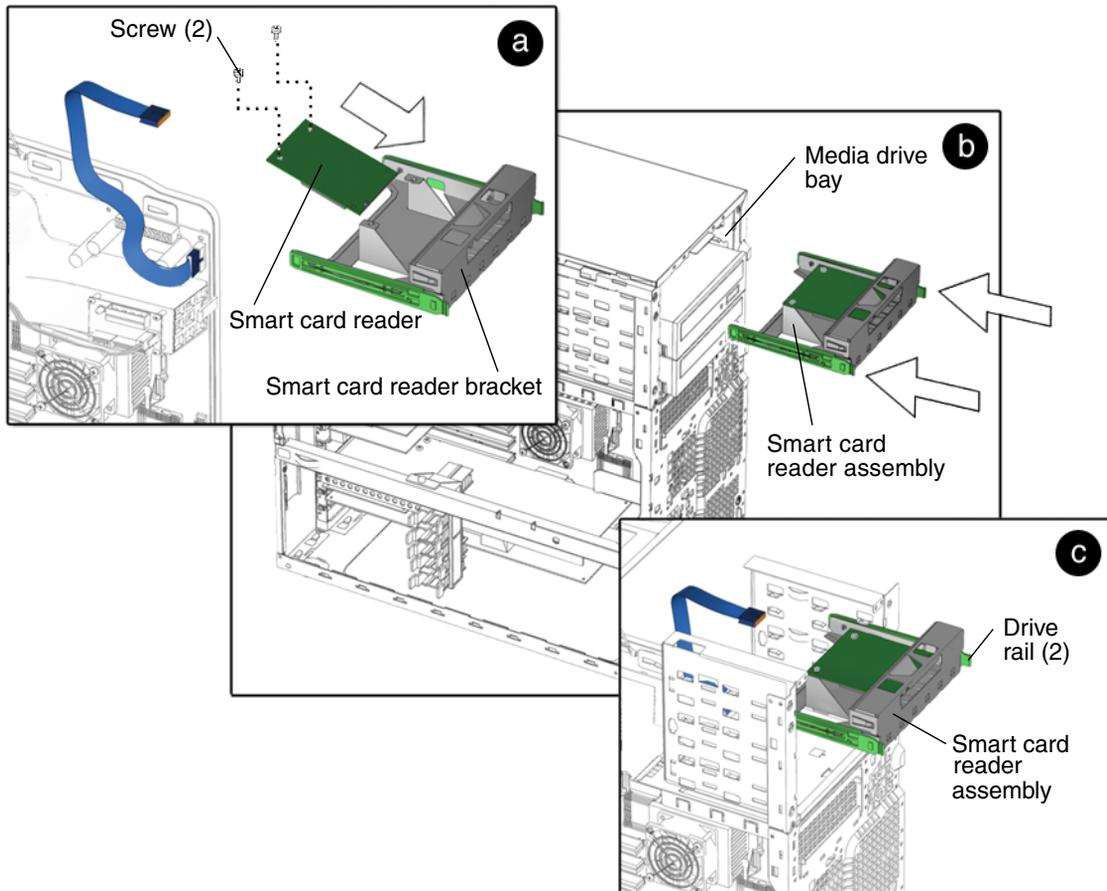
**FIGURE 12-18** Installing the Smart Card Reader
