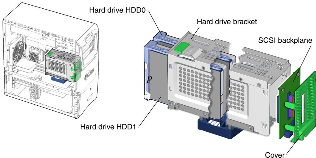
**FIGURE 12-1** Hard Drive Assembly Location and Identification
