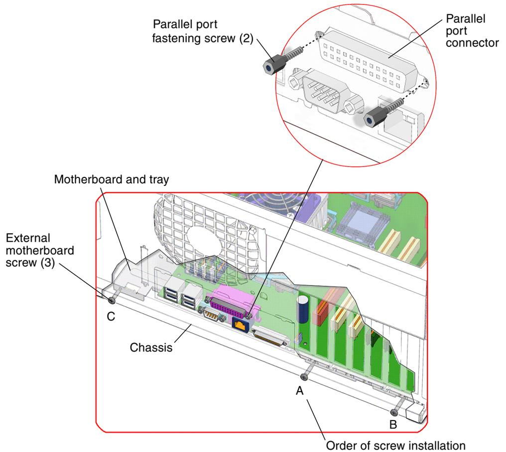
**FIGURE 11-51** Installing the External Motherboard and Parallel Port Fastening Screws
