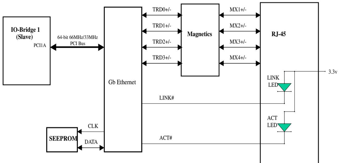
FIGURE C-12 Gigabit Ethernet Block Diagram
