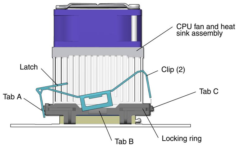
**FIGURE 11-26** Installing the Clip on Tab B
