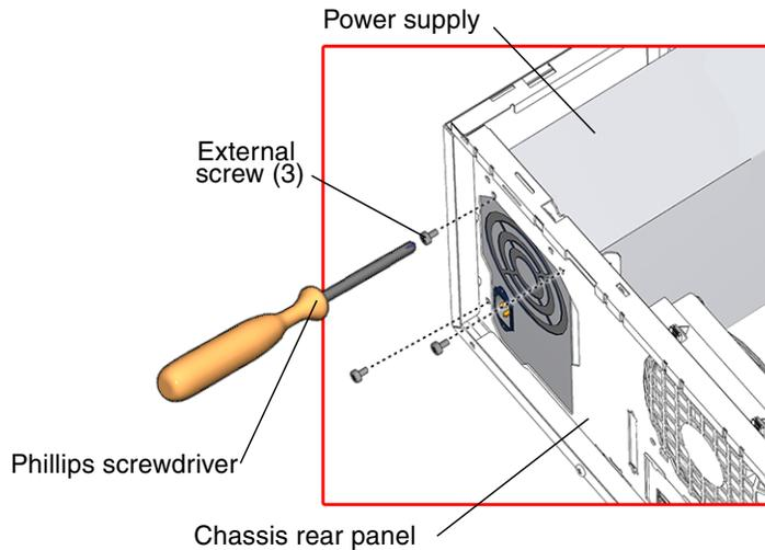
**FIGURE 13-8** External Screws for the Power Supply
