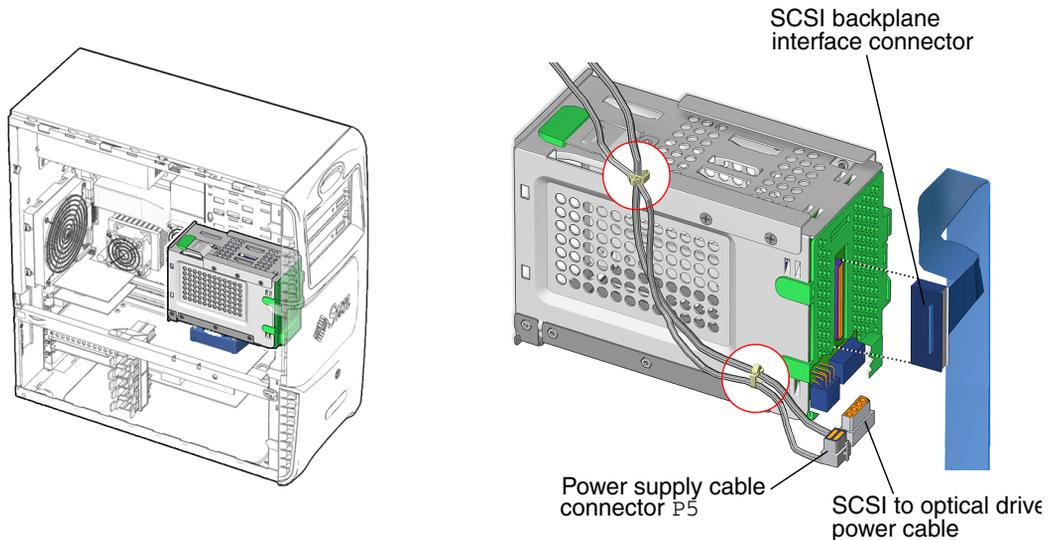
**FIGURE 14-10** Hard Drive Cable Location and Identification
