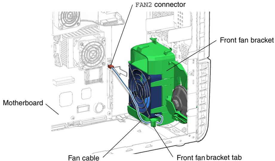
**FIGURE 13-15** Routing and Connecting the Front Fan Cable
