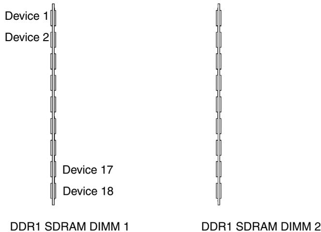
**FIGURE C-7** Bank Interleaving
