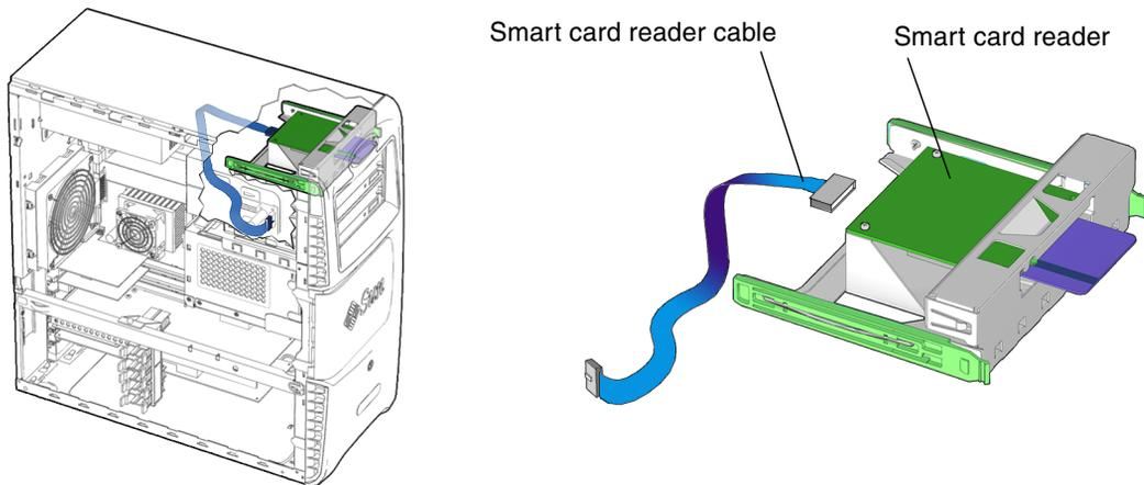
**FIGURE 14-2** Smart Card Reader Location and Identification
