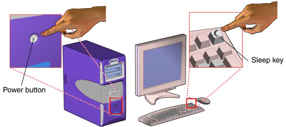
**FIGURE 10-2** Power Button and Sleep Key Location and Identification
