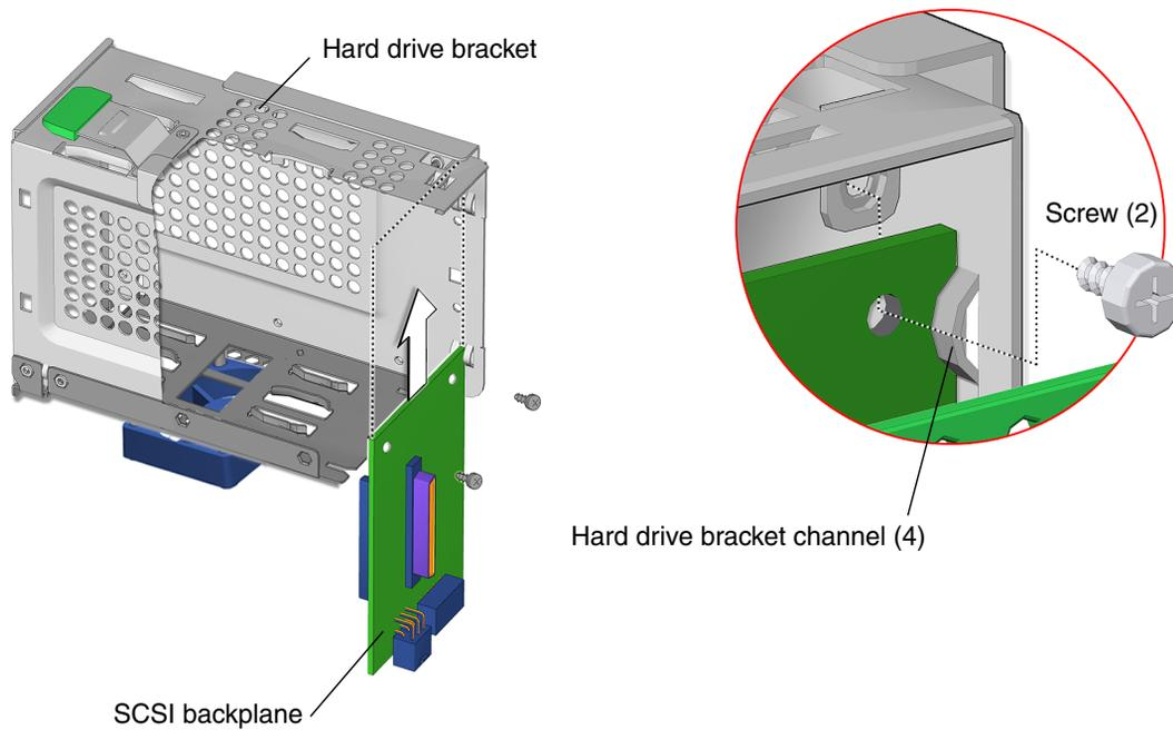
**FIGURE 13-27** Aligning the SCSI Backplane to Hard Drive Bracket
