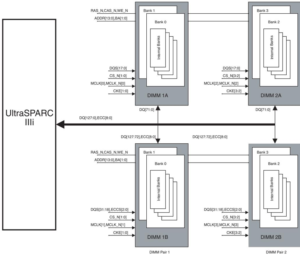
**FIGURE C-4** Memory Subsystem Block Diagram
