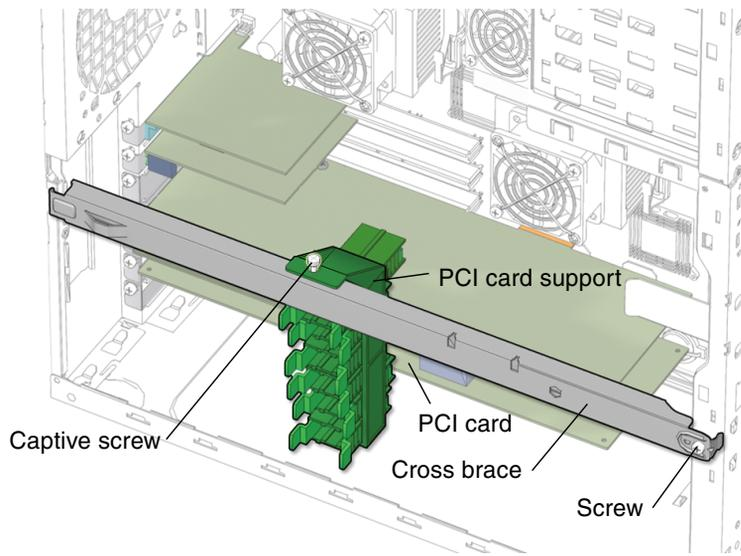
**FIGURE 13-43** Installing the Chassis Cross Brace
