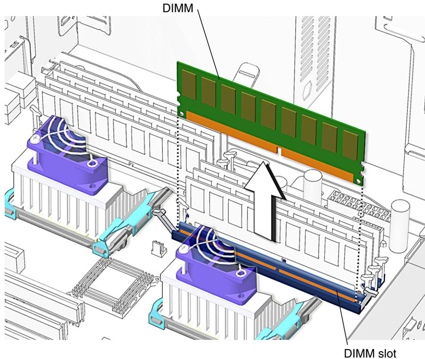
**FIGURE 11-3** Removing the DIMM
