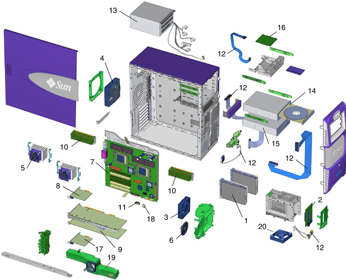
FIGURE 2-4 Exploded Diagram of Sun Blade 2500 Replaceable Components
