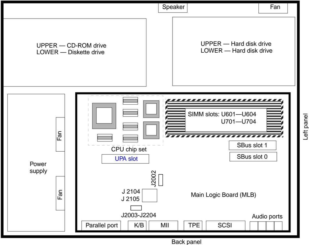
Figure 3-8 Location of the Serial Port Jumpers
