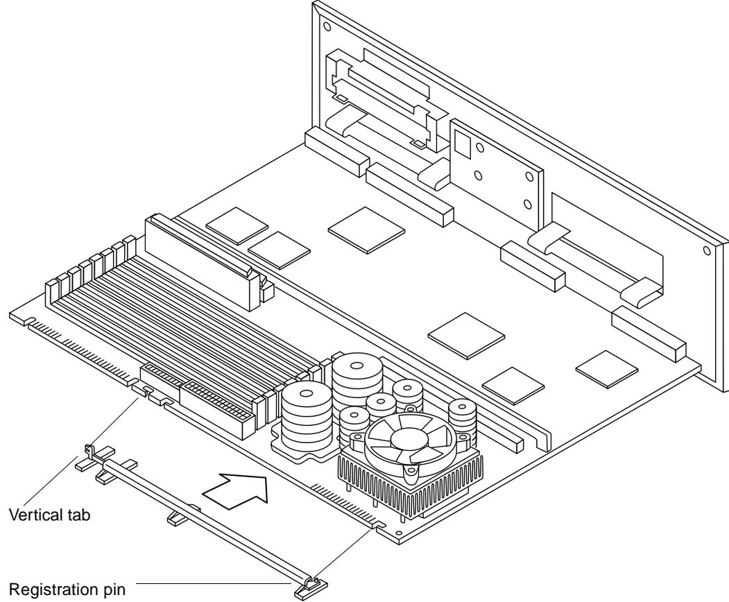
*Figure 3-2* System Motherboard and Front Card Guide.
