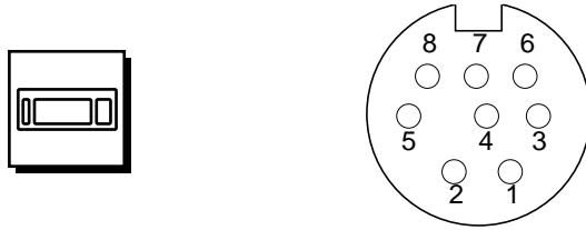
FIGURE B-1 Keyboard/Mouse Connector Pin Configuration
