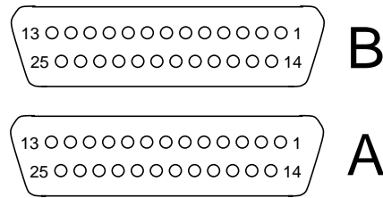
FIGURE 1-2 DB-25 Serial Connectors
