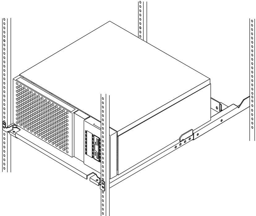
**FIGURE 11** Placing the Ultra 30/60 System in the Rack
