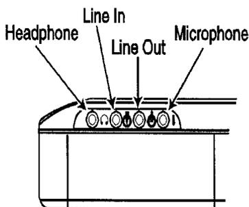
**Figure 2-4 Onboard Audio**
