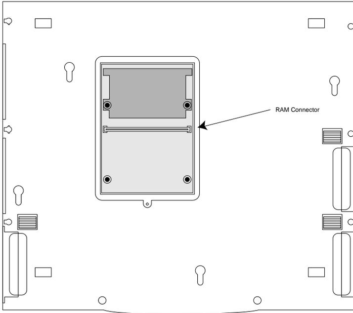
**Figure 1-21 Installing the Memory Module**
