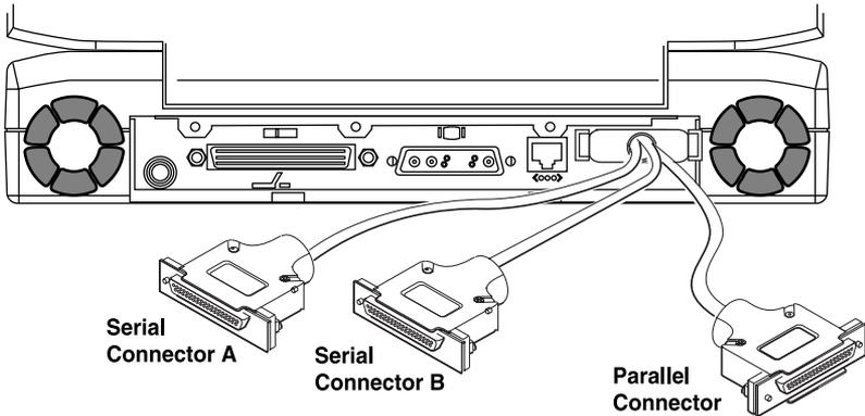
**Figure 1-19 Serial and Parallel Connections**
