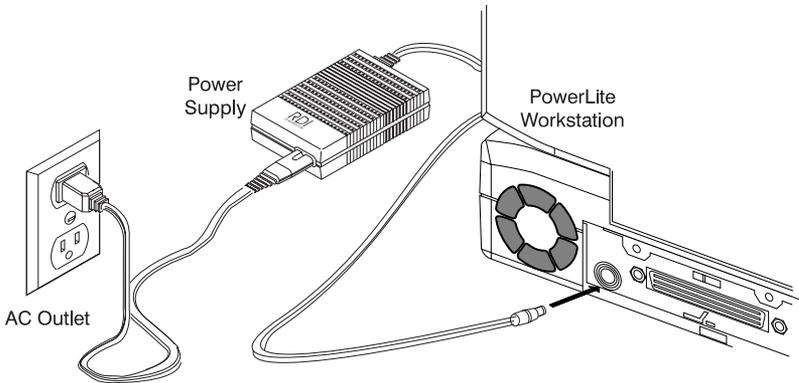
**Figure 1-11 Connecting to AC Power**
