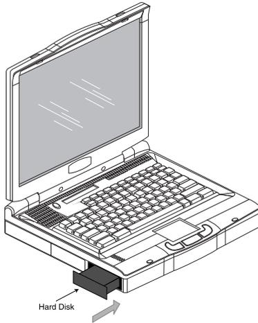
**Figure 1-17 Installing a Hard Disk Drive**
