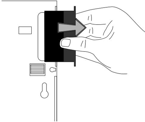
**Figure 1-16 Removing the Hard Disk Drive (cont'd)**
