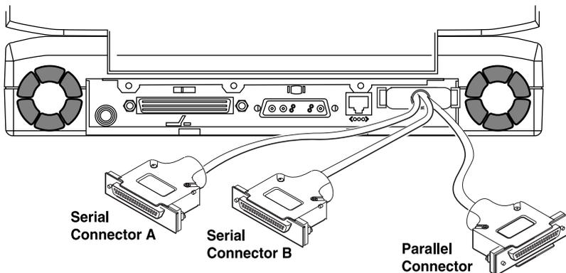
**Figure 1-33 Break-Out Cable Connections**
