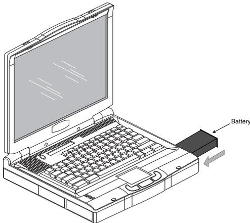
**Figure 1-12 Installing the Battery Pack**
