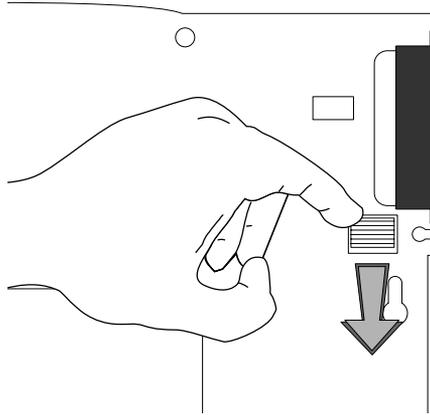
**Figure 1-13 Removing the Battery Pack**
