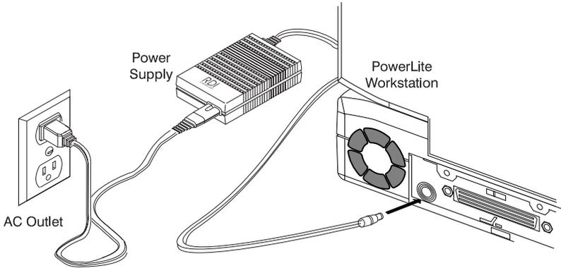
**Step 5 Plug in the AC power adapter.**
