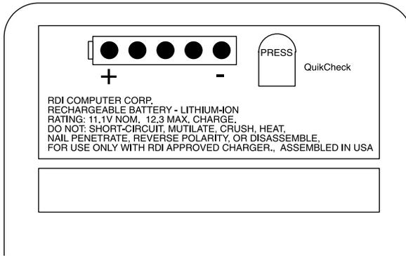
**Figure 1-34 Lithium-Ion Battery Module**
