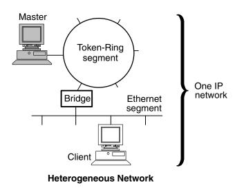
Figure 1. Heterogeneous Network. This illustration shows a single IP network in which the master server uses its token-ring connection and a bridge to communicate with its client on an Ethernet segment.
