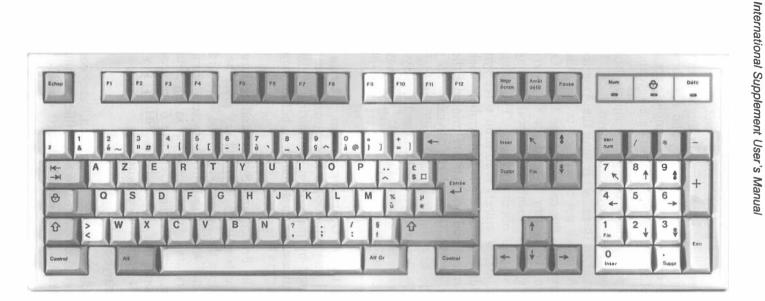
Figure 1. French Personal Computer Keyboard Layout
