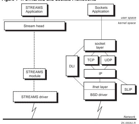
Figure 1-1: STREAMS and Sockets Frameworks
