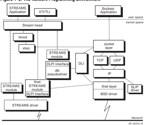
Figure 1–5: The Network Programming Environment
