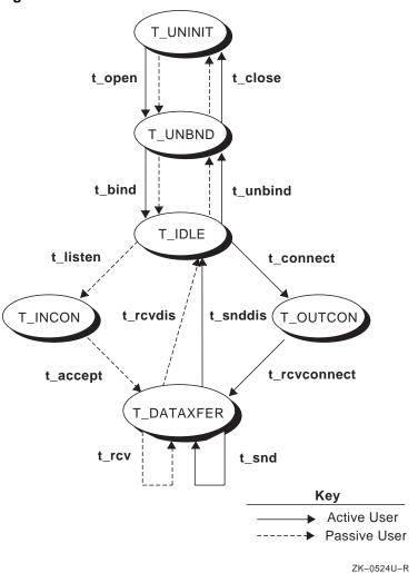
Figure 3-3: State Transitions for Connection-Oriented Transport Services
