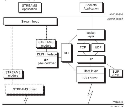
Figure 1–4: Bridging BSD Drivers to STREAMS Protocol Stacks
