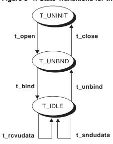
Figure 3-4: State Transitions for the Connectionless Transport Service
