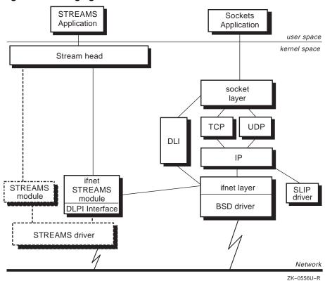
Figure 1-3: Bridging STREAMS Drivers to Sockets Protocol Stacks
