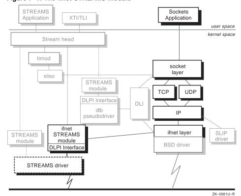
Figure 7-1: The ifnet STREAMS module
