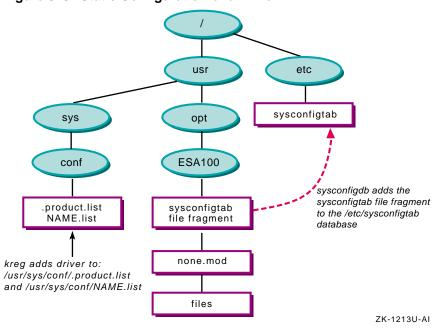
Figure 5-5: Static Configuration of a Driver
