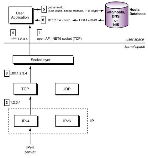
Figure 4–5: Using AF\_INET6 Socket for IPv4 Communications (Receive)
