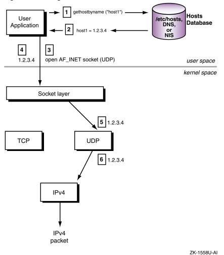
Figure 4–2: Using AF\_INET Socket for IPv4 Communications
