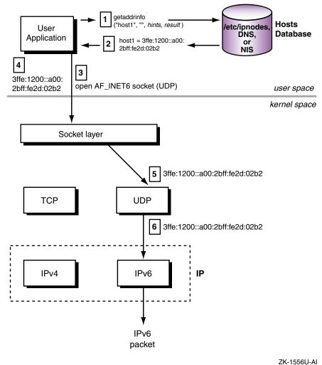
Figure 4–3: Using AF\_INET6 Socket for IPv6 Communications
