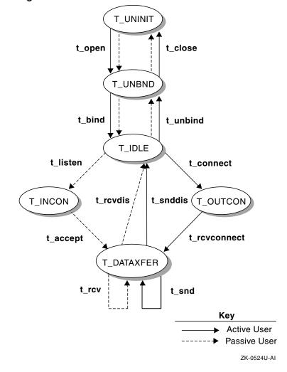
Figure 3–3: State Transitions for Connection-Oriented Transport Services
