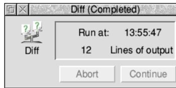
This summary window displays the sprite of the application and the time at which the command was run. The Title bar is the same as for the text window. There are two action buttons, **Abort** and either **Pause** or **Continue**, which allow the program to be aborted, paused, and continued in an identical fashion to the menu on the Text window.
