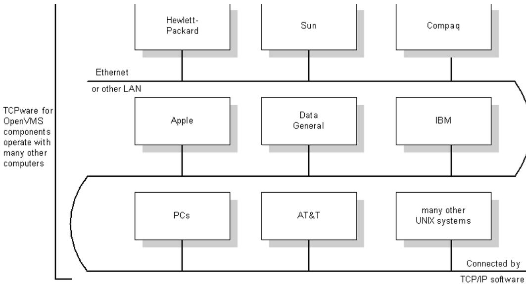
TCPware for OpenVMS components operate with many other computers. TCPware for OpenVMS components also operate with many network support devices that are compatible with TCP/IP, Ethernet, and other local area networks (LANs), as shown in Figure 1-2.
