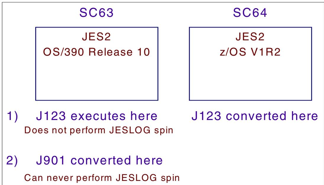
Figure 4-13 Mixed MAS environment and JESLOG spin processing
