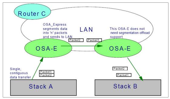
Figure 11-7 Offload segmentations only packets to the LAN
