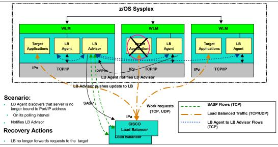
Figure 11-44 Target application fails
