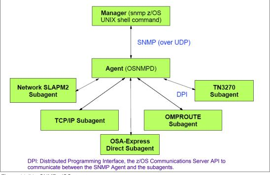
Figure 11-51 shows the SNMP diagram in z/OS.
