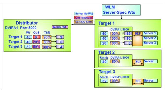
Figure 11-26 Server-specific WLM and sysplex autonomics health monitor for target stack
