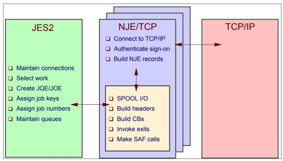
Figure 12-3 Networking address spaces with TCP/IP
