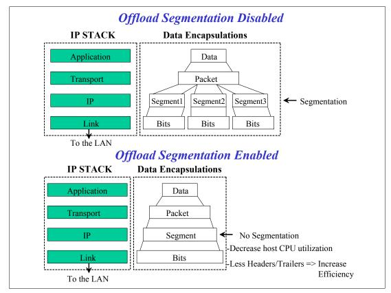
Figure 11-6 Comparative enabled/disabled offload segmentation
