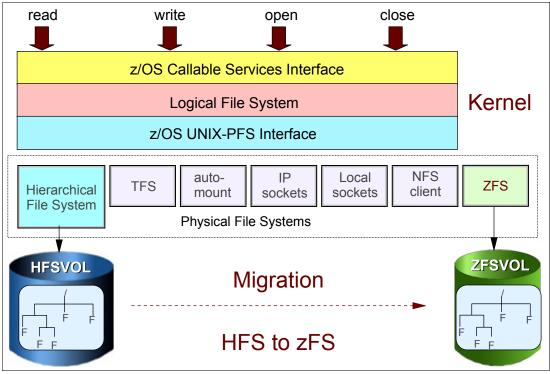
Figure 9-1 z/OS UNIX communication between LFS and PFS
