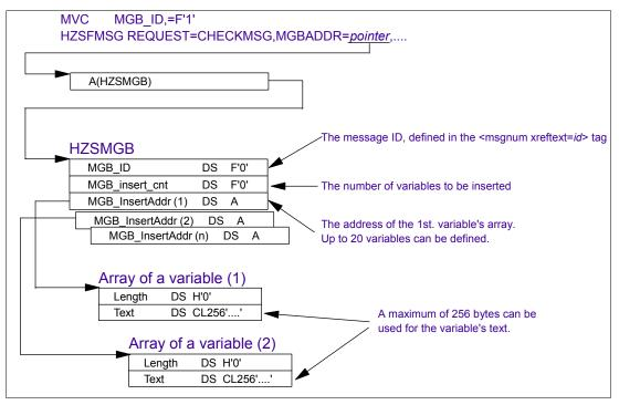
Figure 8-20 The HZSMGB control block
