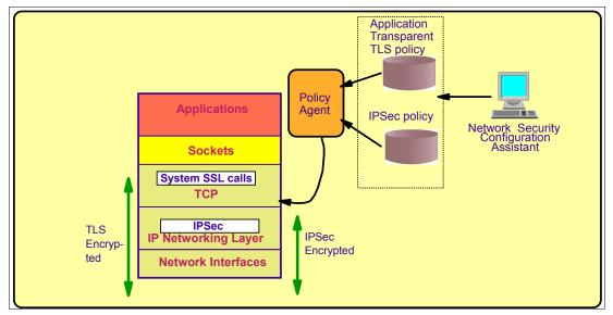
Figure 11-70 shows the IP stack and the TLS/SSL service.
