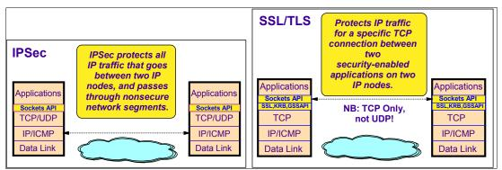
Figure 11-63 IPSec / SSL and TCP/IP stack relation.
