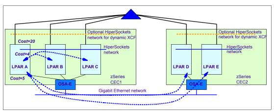
Figure 11-12 TCP/IP sysplex improved distribution optimized routing with V1R7
