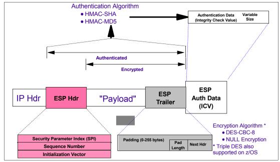
Figure 11-69 Encapsulating security payload headers.
