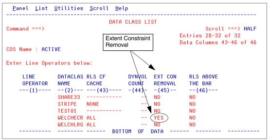
Figure 10-14 Extent Constraint Removal attribute on the DATACLAS definition
