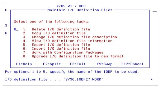
Figure 2-9 HCD panel to upgrade an existing IODF to V5 level
