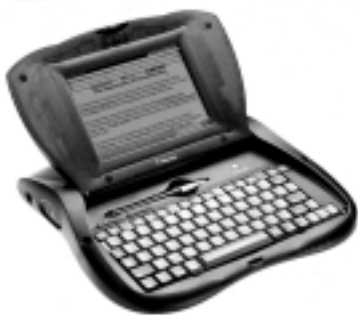
Although it looked like a futuristic PowerBook, the eMate 300 was essentially a Newton with a built-in keyboard.
