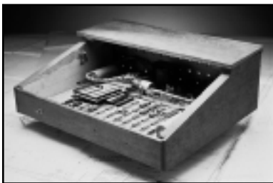
The original Apple I (shown here in a custom-built wooden case) was little more than a circuit board to which customers were expected to add a case, power supply, monitor, and keyboard.
