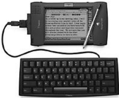
The MessagePad 2000 was notably faster than its predecessors thanks to its 160MHz StrongARM processor.
