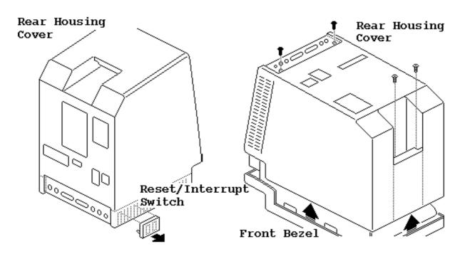
Using a small screwdriver, pry off the reset/interrupt switch on the left side of the case.
