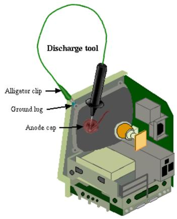
If you are working on a compact Mac that contains a CRT (just like SE/30) and incorrectly discharge the CRT to the metal chassis, you may destroy the logic board.
