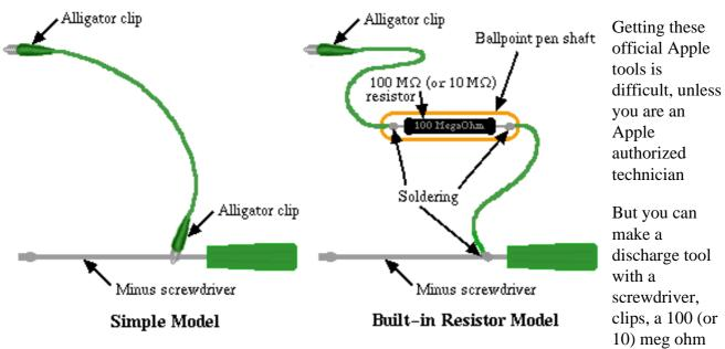
resistor, a ballpoint pen shaft (the outer tube of a ballpoint pen) and some wires. Insulating the resistor and its leads with the ballpoint pen shaft prevents careless short between the anode and other components.
