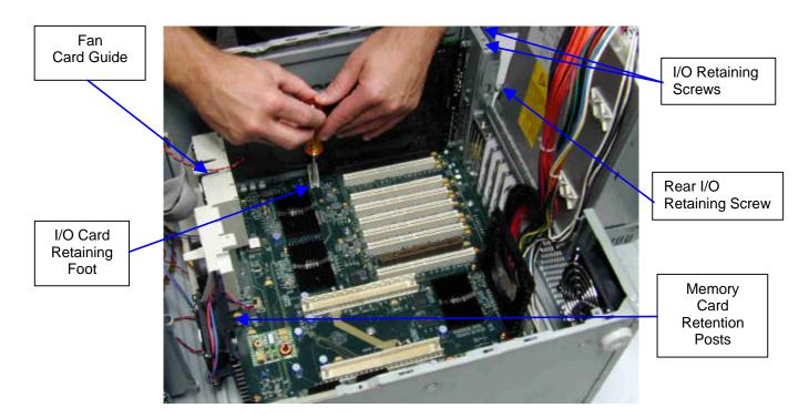
Figure 45. Internal Component Locations
