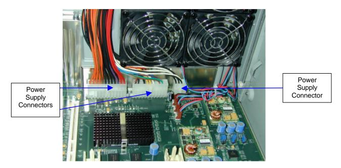
Figure 48. Main Power Connection
