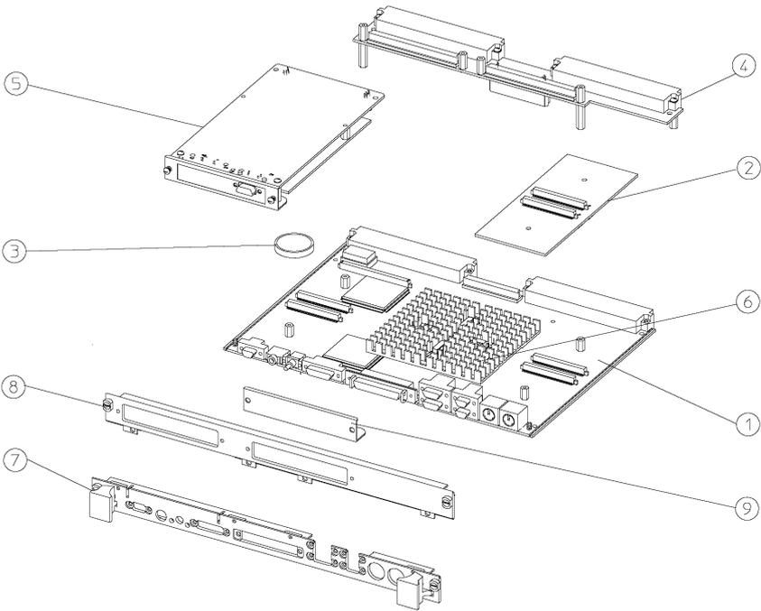
**Figure 5-1**                      **Model 743 Board Computer Exploded View**
