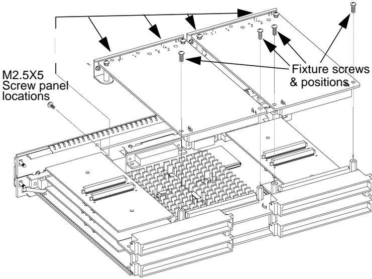
**Figure 5-4 GSC Fasteners**
