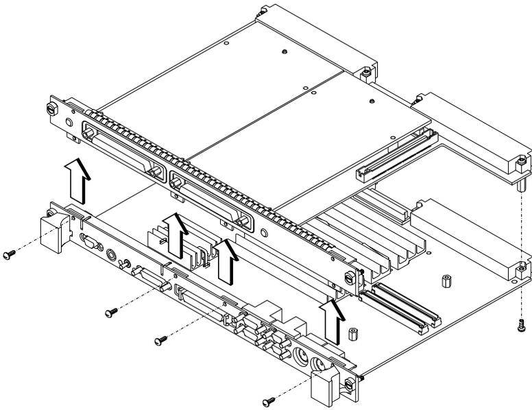
Figure 5-10 Removing the PMC Bridge Adapter
