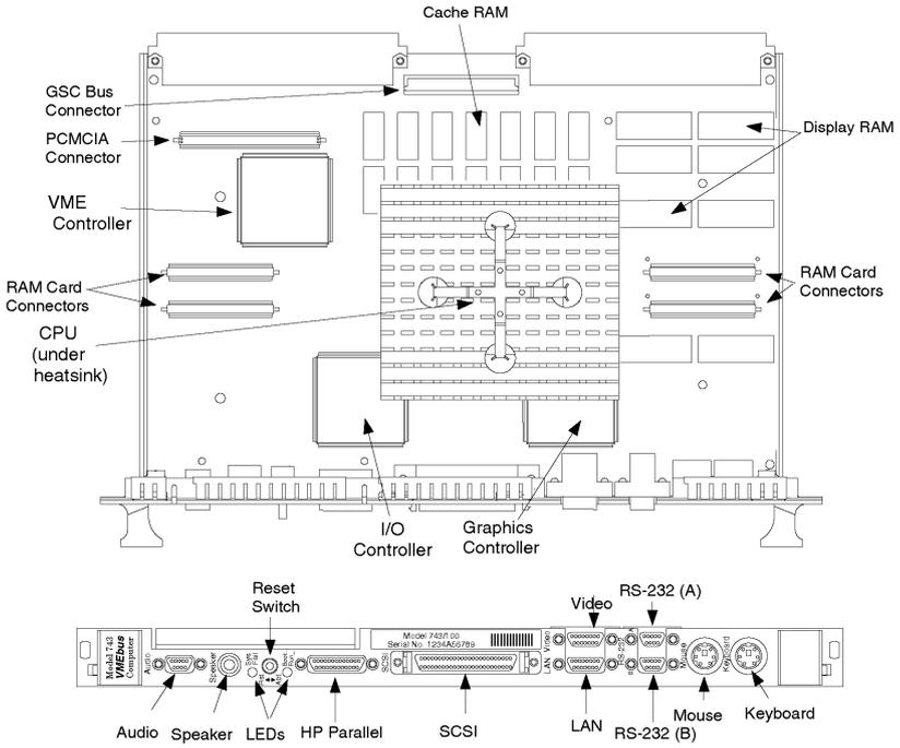
**Figure 2-1** Model 743 VMEbus Board Computer
