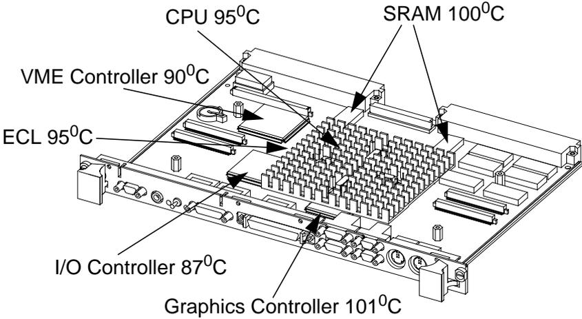
**Figure 1-1 Model 743 VMEbus Board Computer Temperatures**
