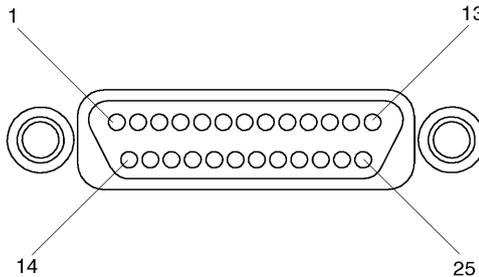
**Figure 2-4 HP Parallel Connector**
