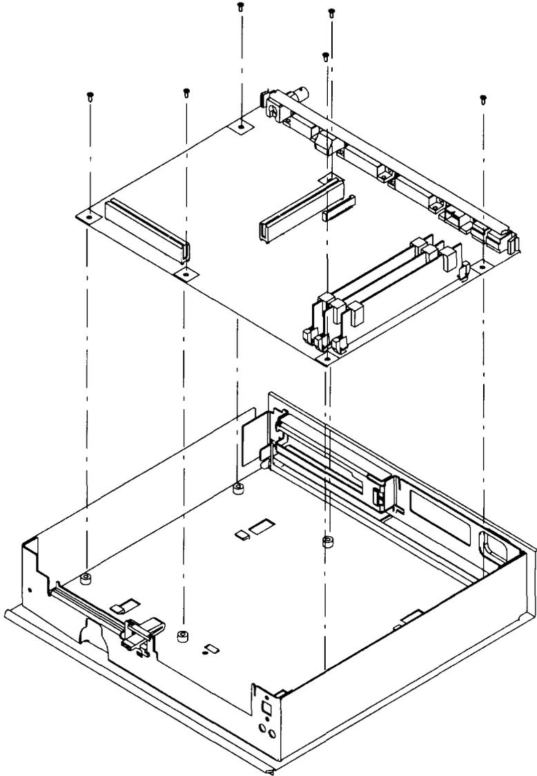
9. Lift the system board assembly up and out of the chassis.
