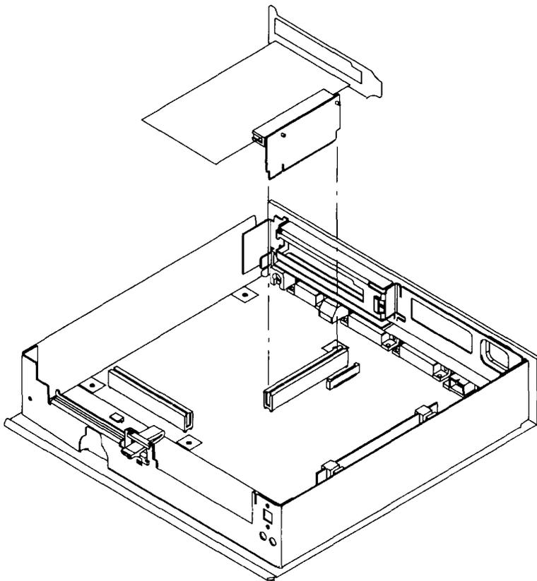
4. Separate the PCI adapter from the riser card.
