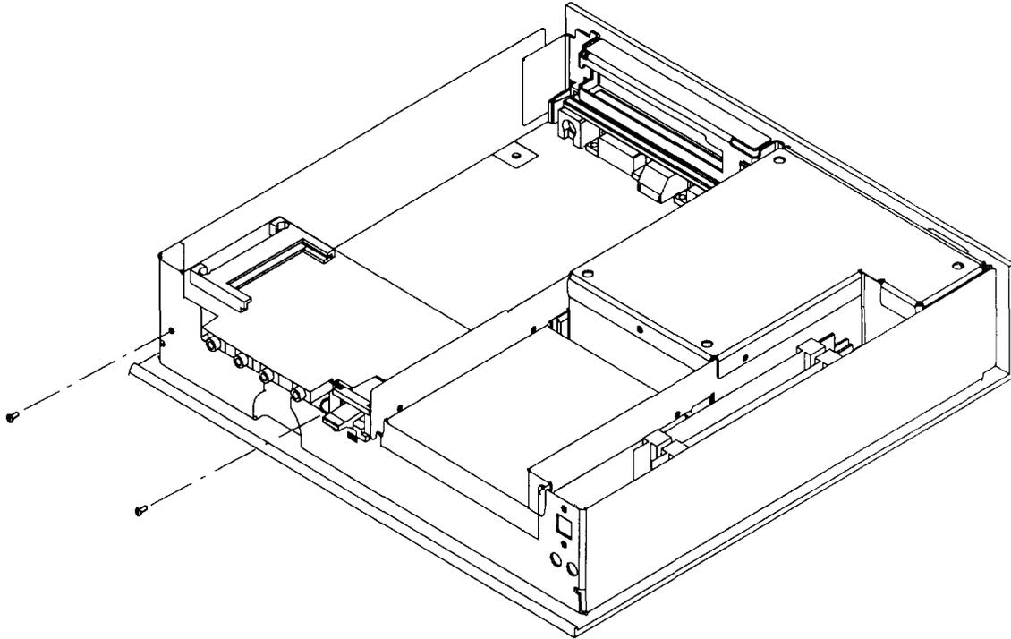
4. Remove the blank cover plate in the Xstation cover and replace it with the new Business Audio card cover plate.
