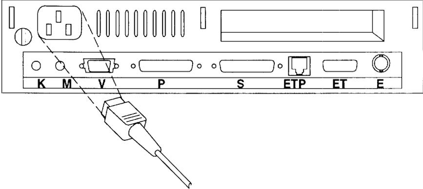
**Note:** Be sure to connect the power cord to an electrical outlet that is easily accessible. To completely remove power, you must disconnect the power cord from the outlet.
