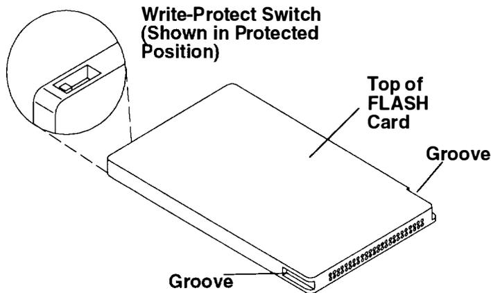
2. Turn the FLASH card so that the sockets face the pins in the FLASH card connector.
