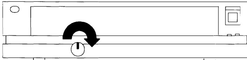
4. Open the cover door, then lift and hold the cover latch and slide the cover forward until the cover moves past the latch.
