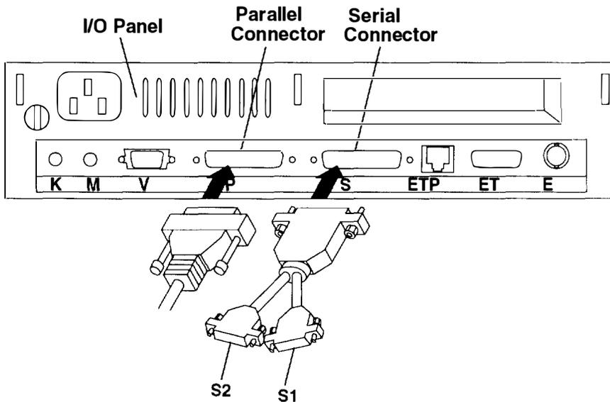
7. Place the display close to the Xstation system unit and plug the display cable into the Xstation I/O panel as shown. Some displays only need the RGB BNC-style connectors. If the display is rolling or is unreadable, disconnect the horizontal (white) and vertical (black) connectors.
