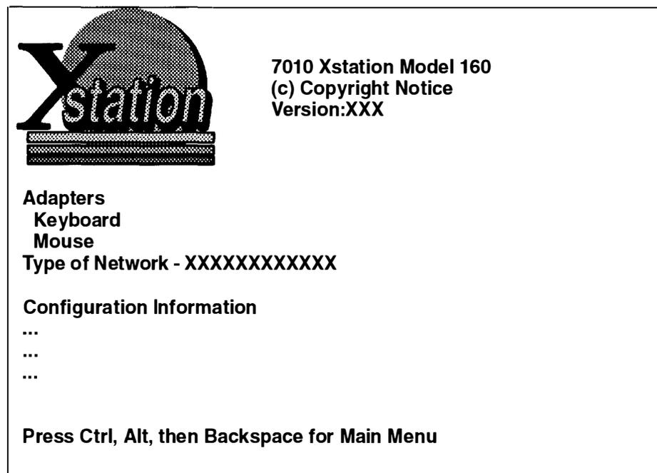
If the Xstation fails to complete the POST or LAN communications test, go to Chapter 5, "Problem Determination Procedures."
