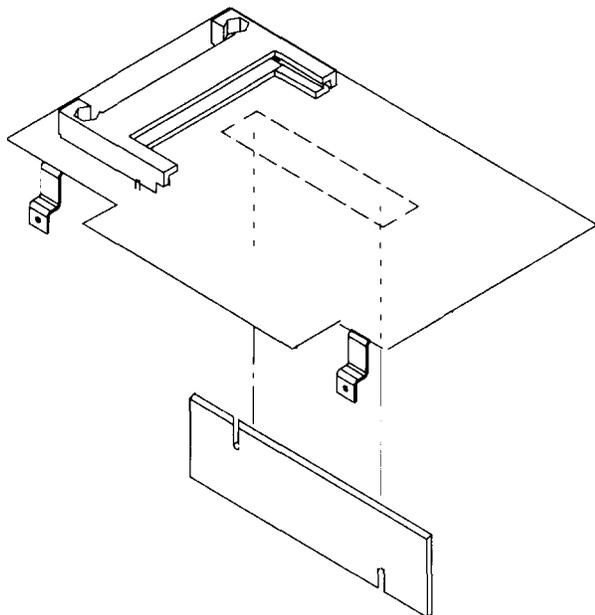
2. Insert the riser card and FLASH connector card into the PCMCIA connector (J4) on the system board
