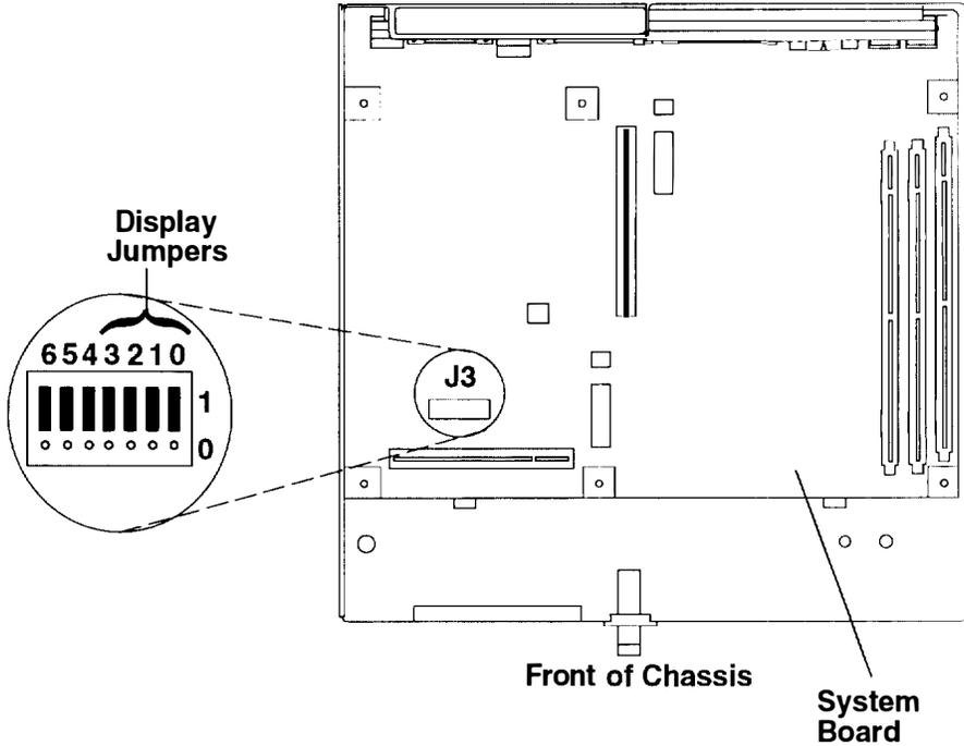
These four jumpers are factory-set to 1111. To change the displays jumper setting, look up the proper setting in the table below, then record that setting here when you configure the system jumpers inside your Xstation.
