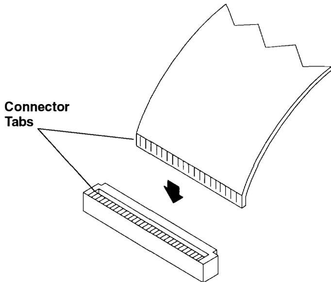
9. Press the connector edge firmly down to lock the cable in place. Ensure that both ends of the cable tab are locked.
