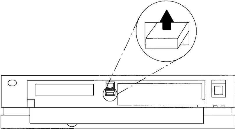
5. Slide the cover to the front, then lift it off the Xstation.
