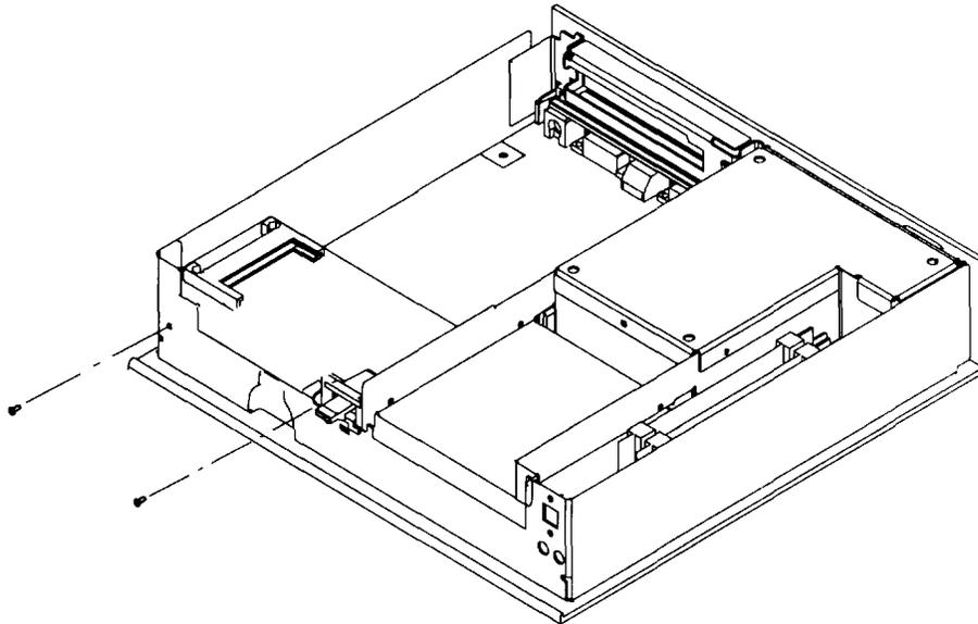
3. Remove the riser card and FLASH connector card from the PCMCIA connector (J4) on the system board
