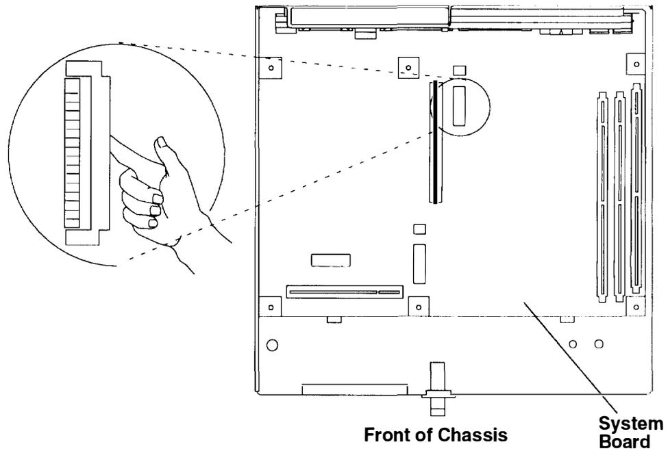
8. Insert the end of the diskette drive cable into the system board connector. The connector tabs on the cable must mate with the connector tabs on the system board connector.
