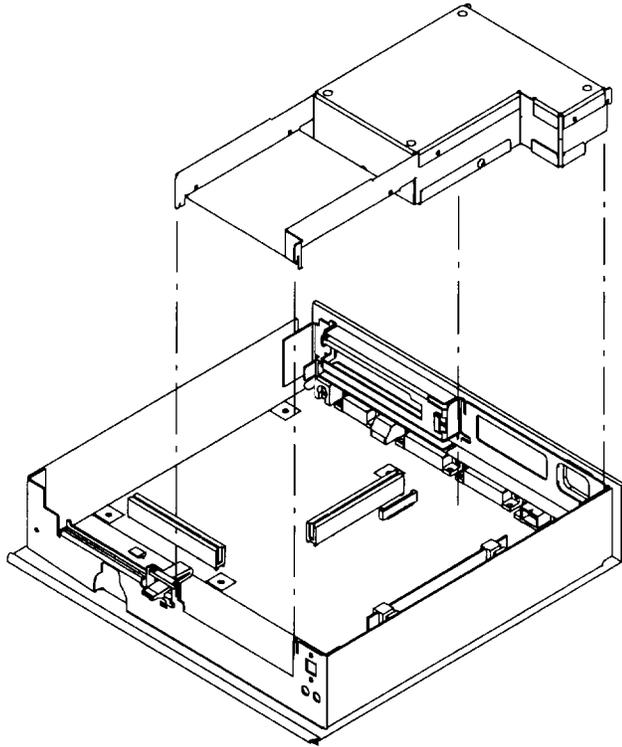
5. Place the drive into the power supply tray. The connector must be toward the rear.
