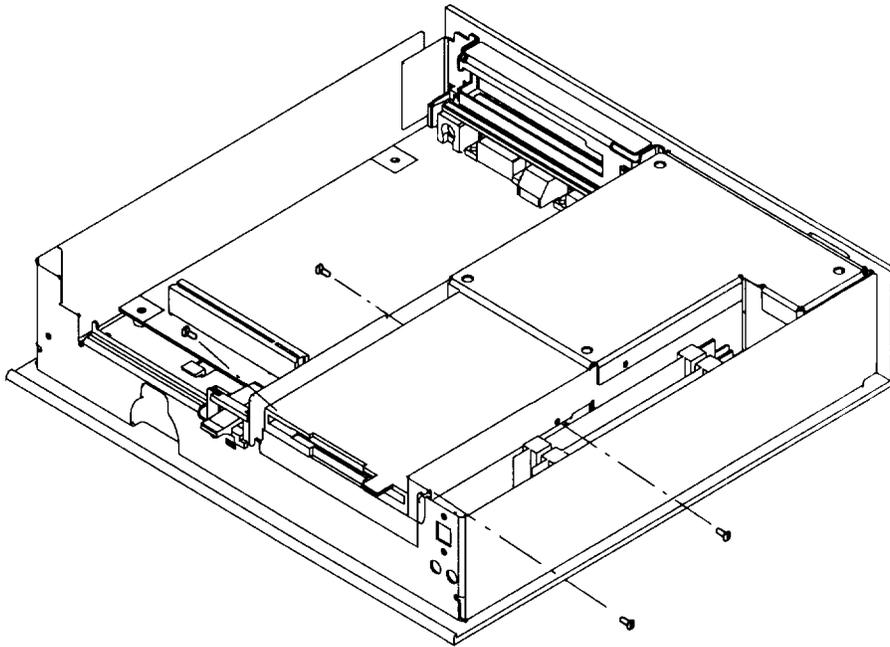
5. Remove the diskette drive from the power supply tray.
