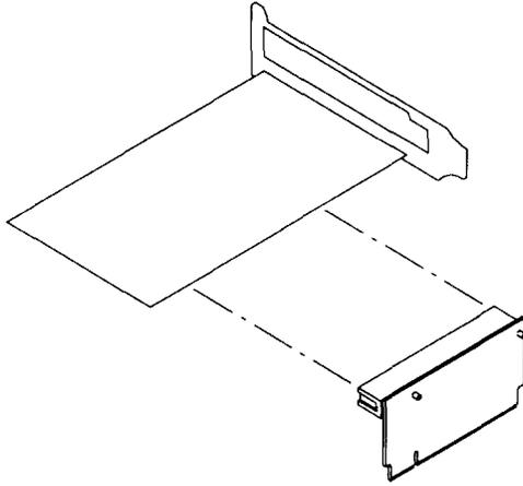
To replace the PCI adapter, perform removal steps in reverse order.
