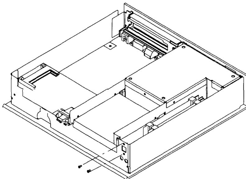
4. Remove the power switch assembly.
