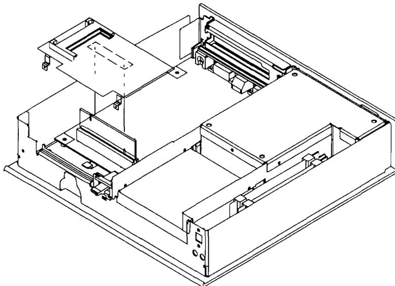
4. Separate the FLASH connector card from the riser card.
