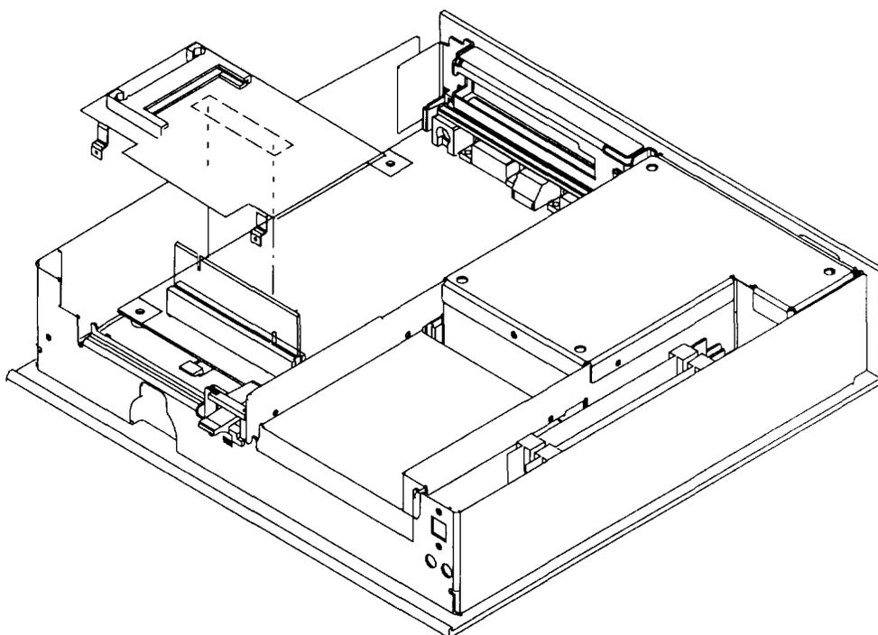
3. Install the two screws into the FLASH connector card brackets.
