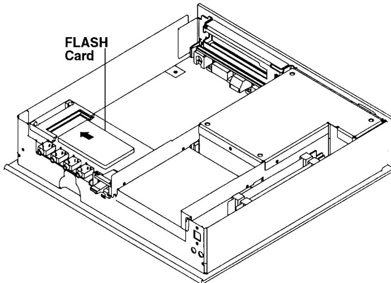
3. Insert the FLASH card into the FLASH card connector on the PCMCIA card.
