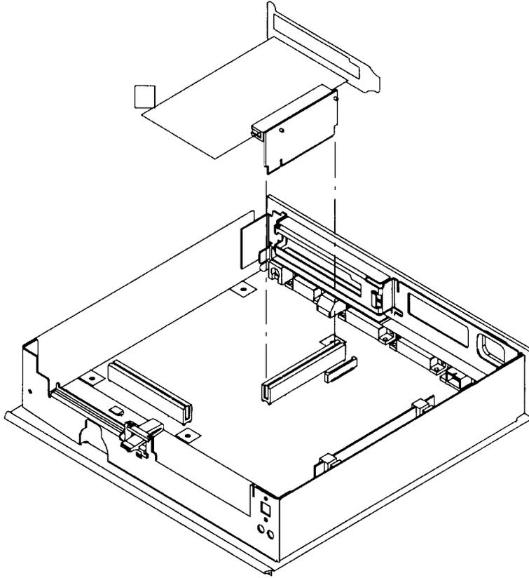
5. Insert and tighten the adapter screw.
