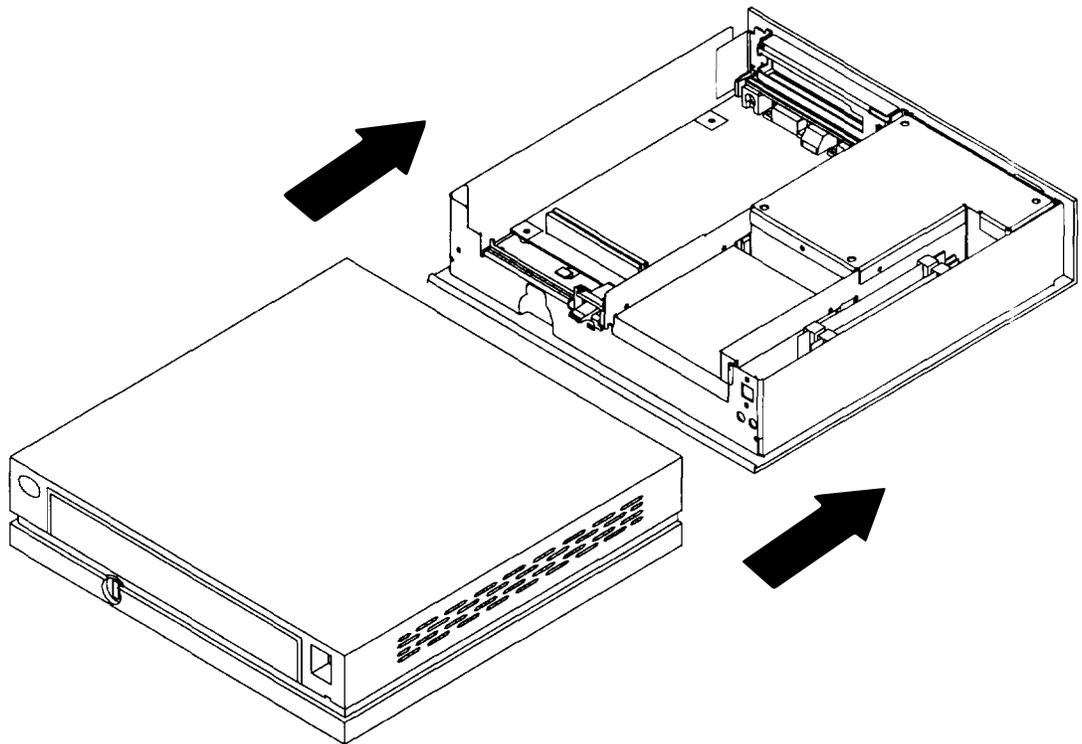
**Note:** If you cannot get the covers on completely, make sure that the drive tray and front of the adapter are properly lined up with cover openings.
