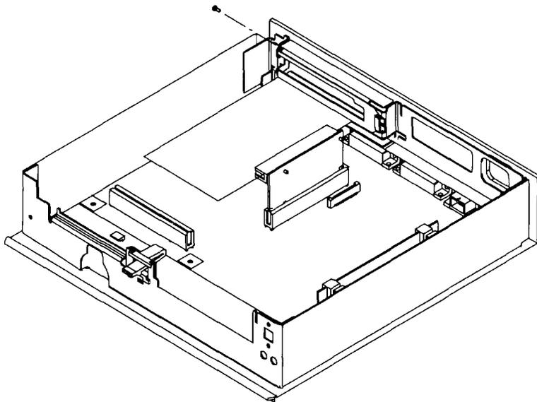
3. Remove the PCI riser and PCI adapter from the PCI connector (J10) on the system board.
