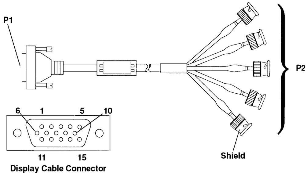
For displays 5081-01x, 6091-0xx, and POWERdisplays 16 and 19, use display cable 58F2901:
