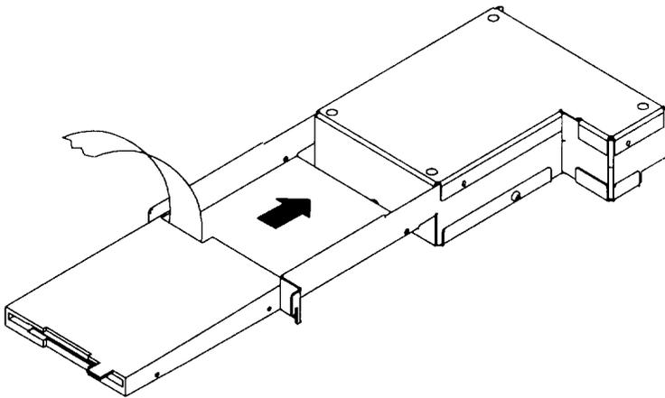
6. Install the four mounting screws into the diskette drive.
