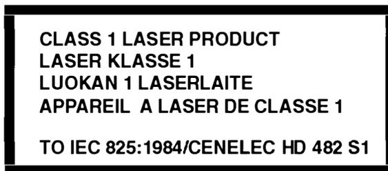
Figure 3. Class 1 System Information Label Required by the IEC 825 Standard
