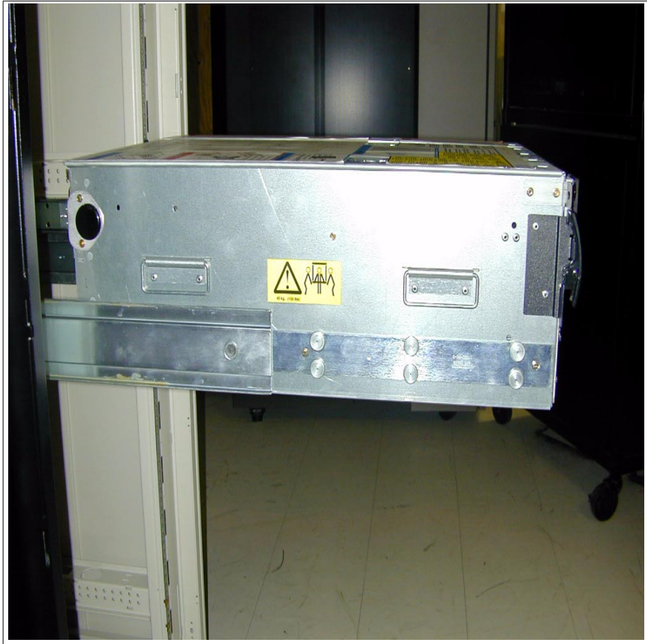
Figure 3-19 System drawer in service position
