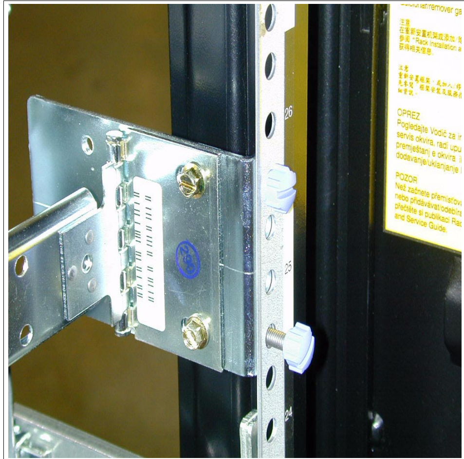
Figure 3-27 Cable management arm rack mounting plate
