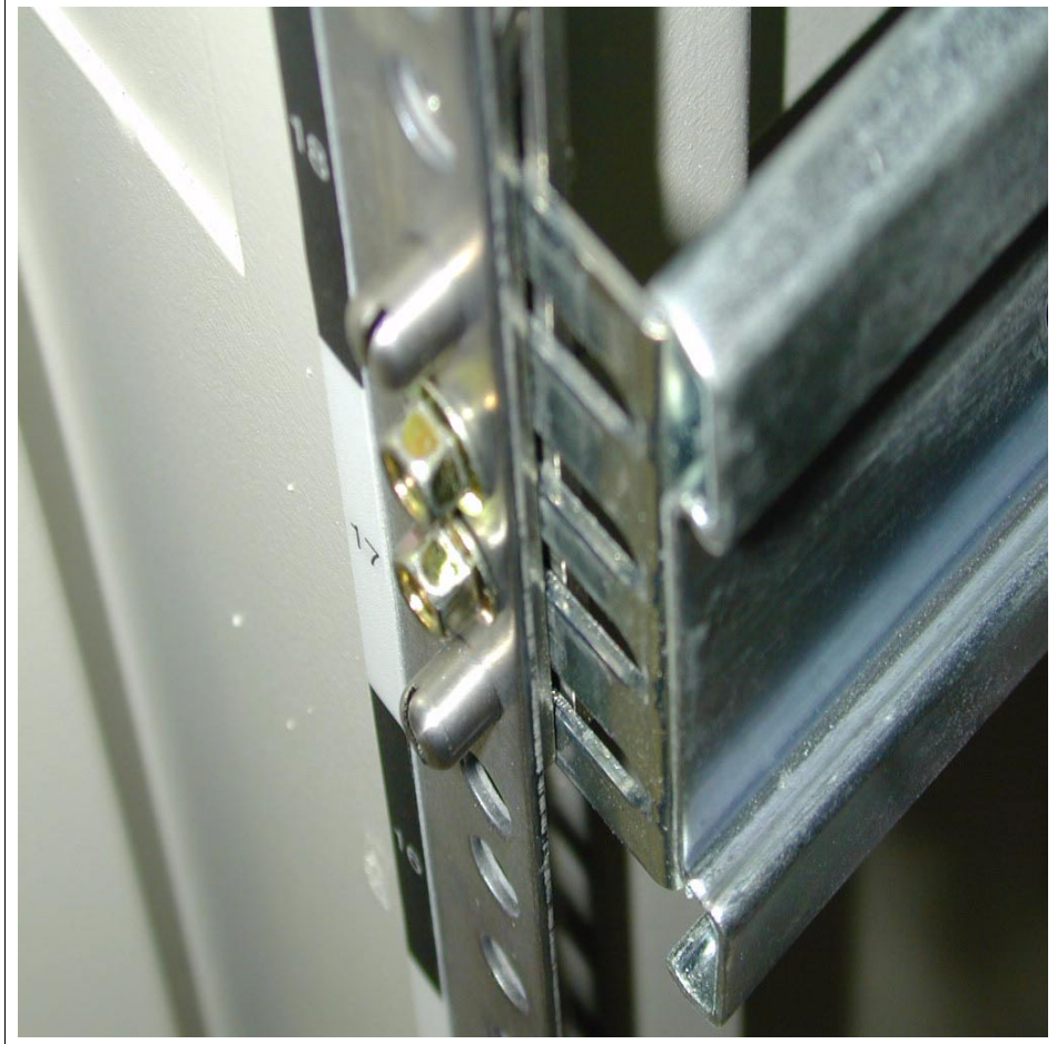
Figure 3-14 Positioning front of rail into rack mounting plate
