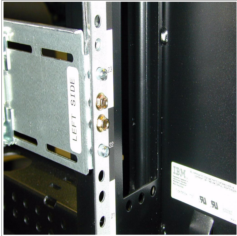
Figure 3-13 Rear rail pin in noted hole location
