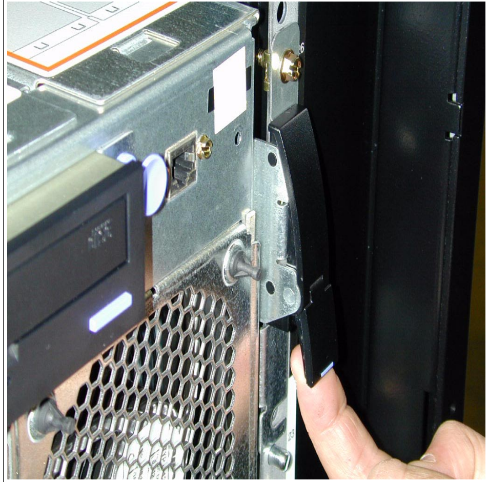
Figure 3-22 Lower section of release latch
