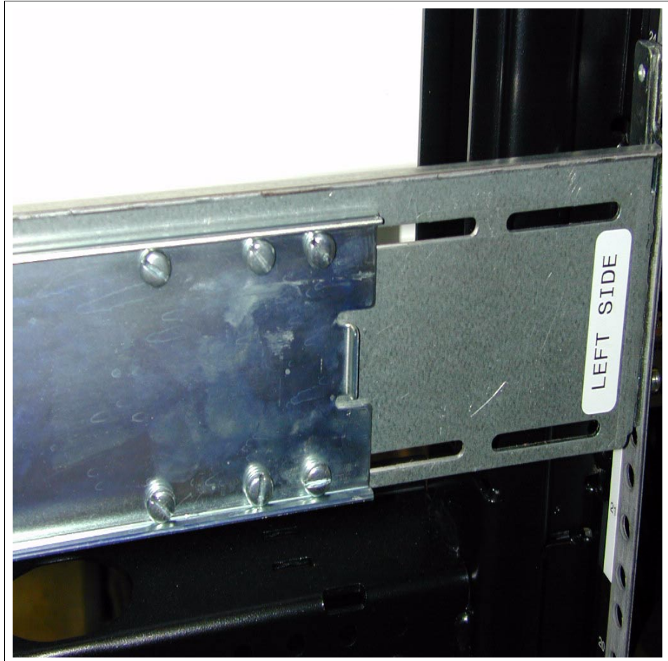
Figure 3-11 Rail length adjustment screws
