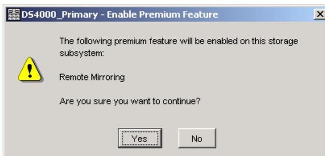
Figure 8-19 Enable Enhanced Remote Mirroring premium feature: Confirmation
