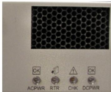
Figure 3-25 Power supply fan LEDs
