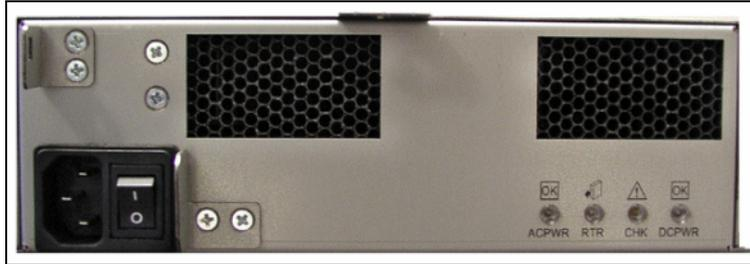
Figure 3-8 Power supply fan LEDs
