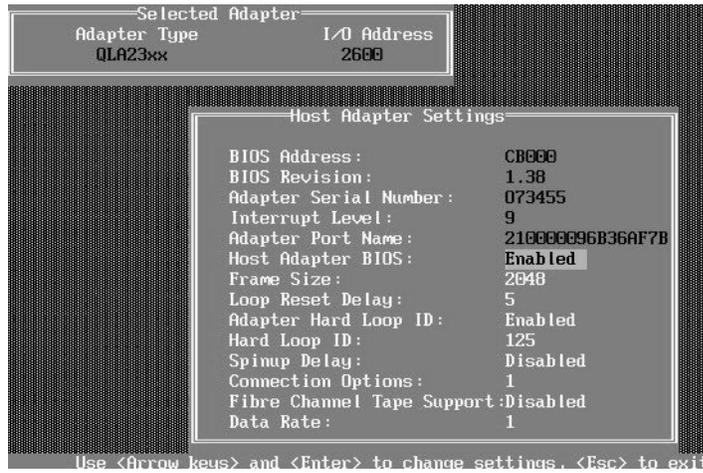
Figure 10-39 Enable host adapter BIOS
