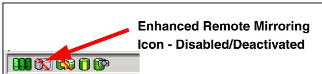
Figure 8-18 Enhanced Remote Mirroring feature icon: Disabled/deactivated
