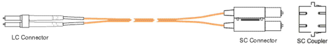
FIGURE 1. LC and SC Fiber-optic Connectors with SC Coupler. The Lucent LC has a form factor about half the size of the SC connector, and uses an insertion release mechanism similar to those on telephone plugs.
