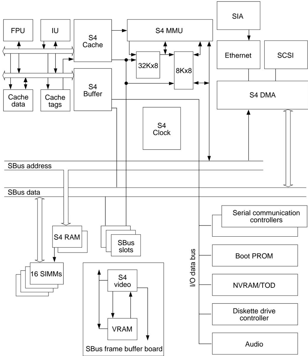
Figure 1-4 A Block Level Diagram of the Main Logic Board
