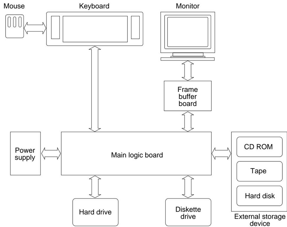
Figure 1-1 SPARCstation 1 and SPARCstation 1+ Block Diagram
