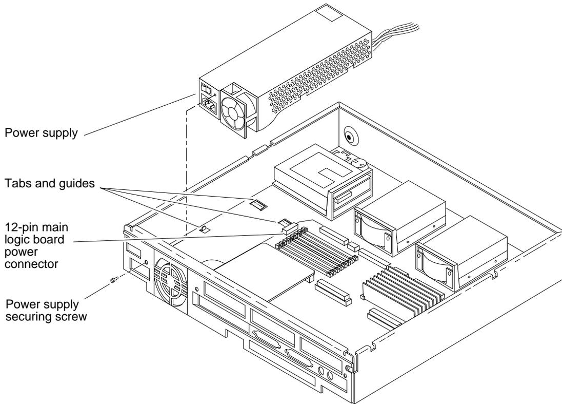
Figure 4-5 Removing and Replacing the Power Supply
