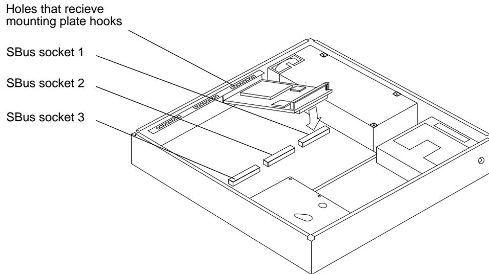
To install an SBus board in the system unit:
