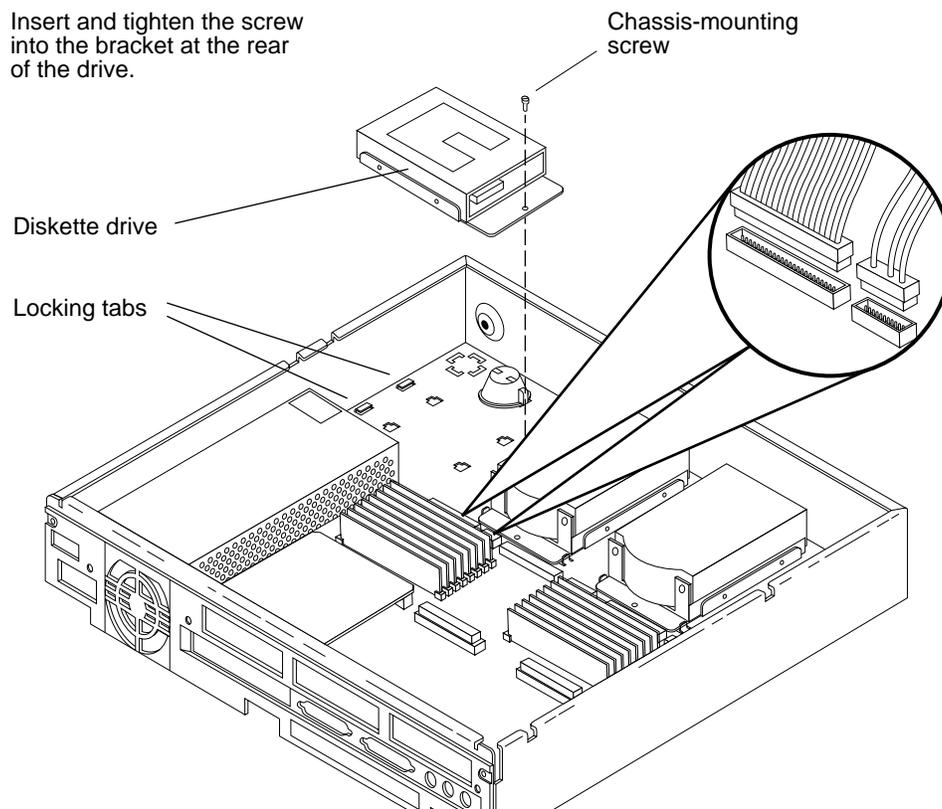
Figure 4-13 Removing and Replacing the Diskette Drive With a Metal Bracket
