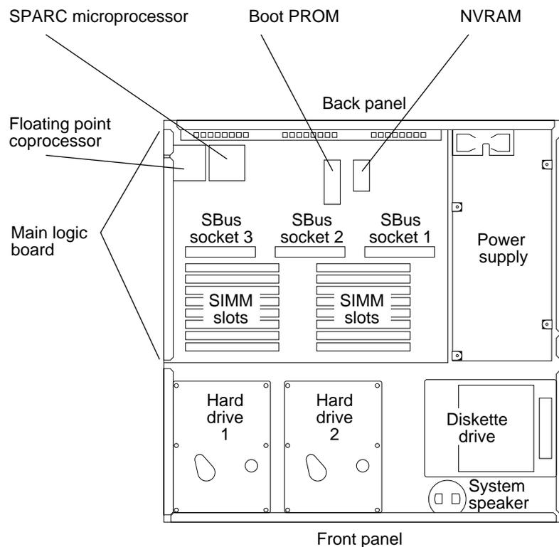
Figure 3-2 System Unit and Subassemblies
