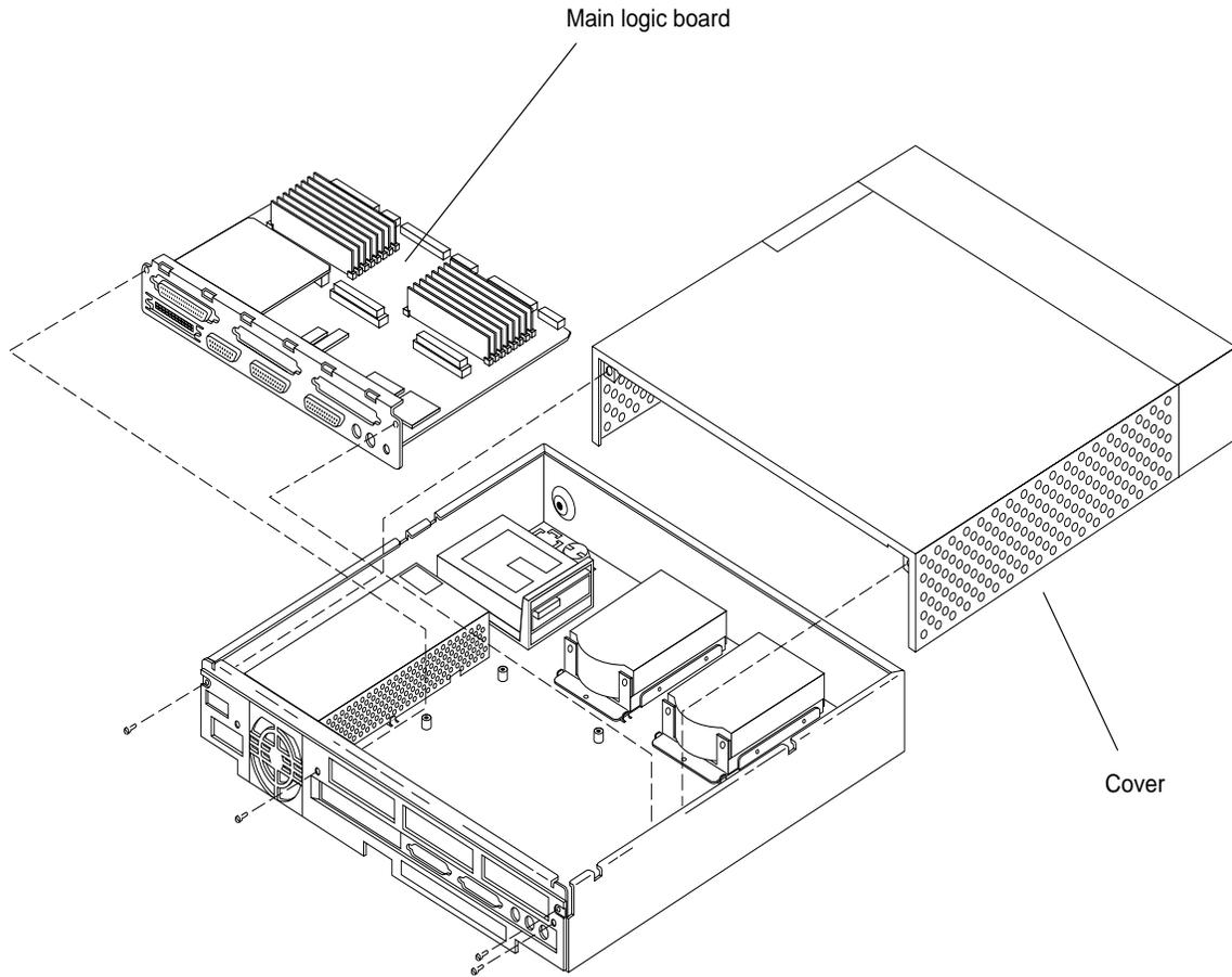
Figure B-3 Exploded View of the System Unit , Sheet 2
