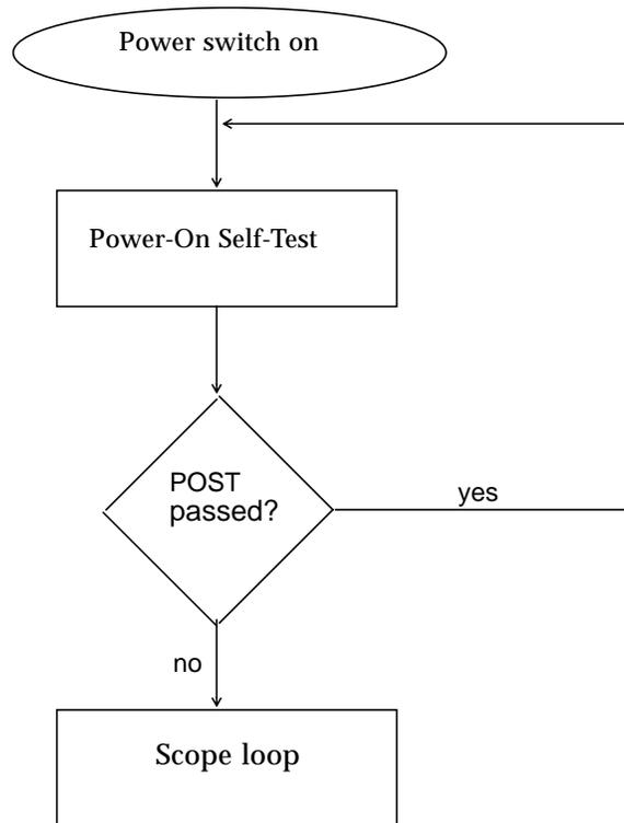
Figure 2-3 Flowchart Illustrating Manufacturing Diagnostics
