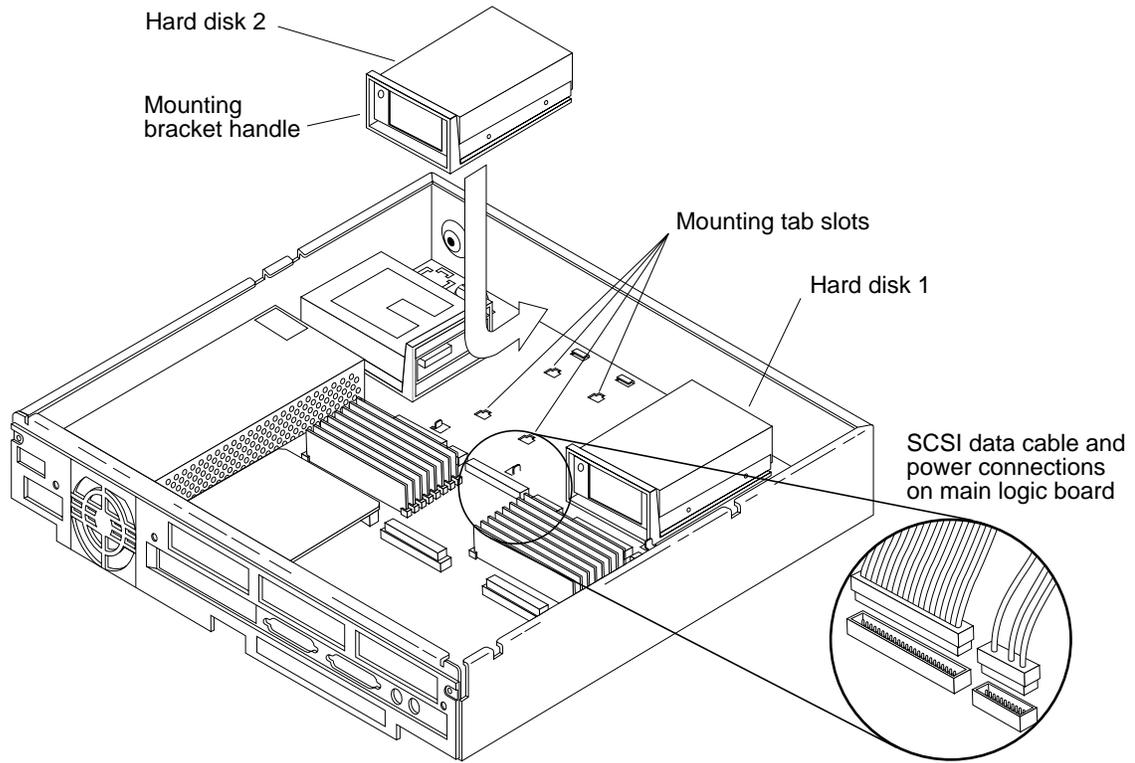
Figure 4-9 Removing and Replacing the Hard Disk Drive With the Plastic Bracket
