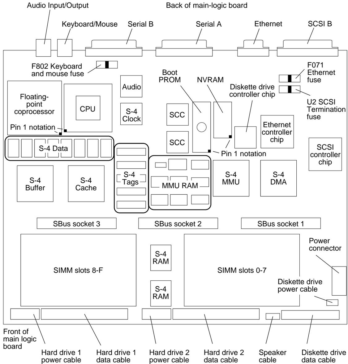
Figure 1-3 The Main Logic Board
