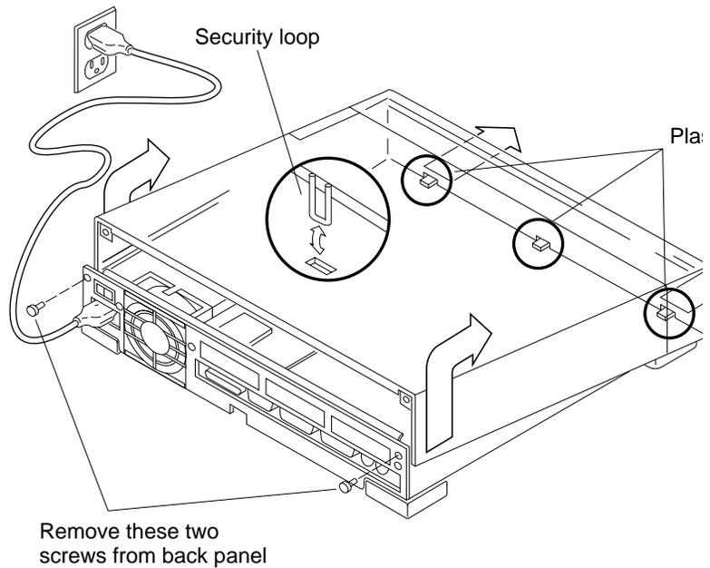
Figure 3-1 Removing the Cover Panel
