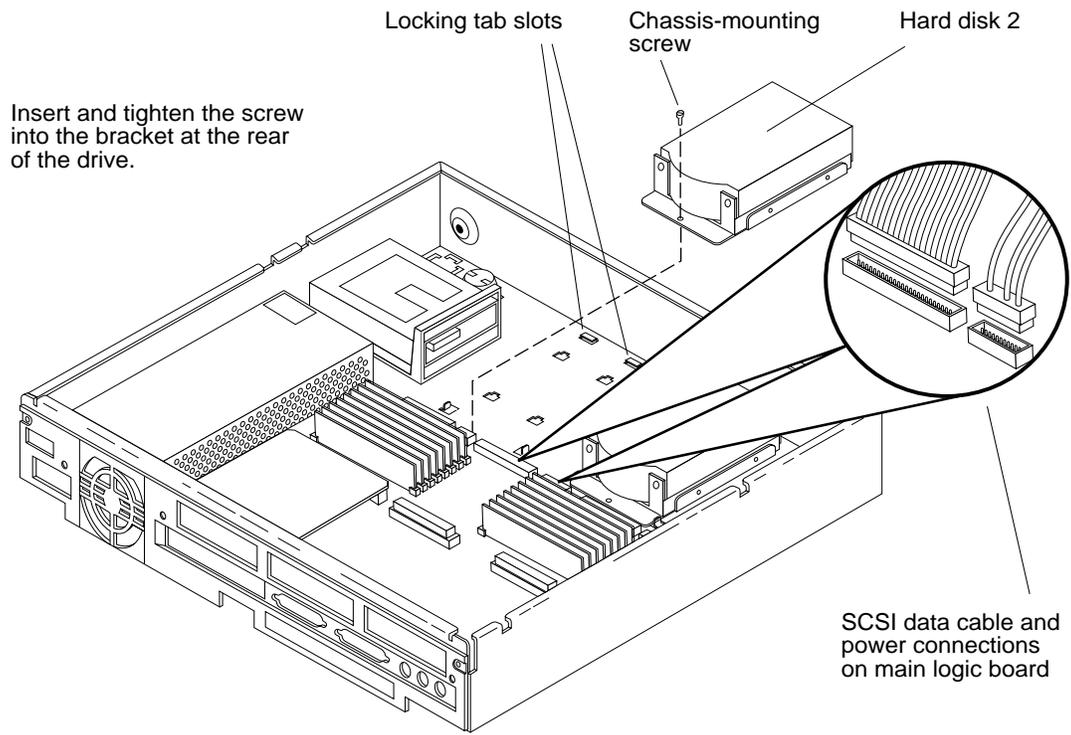
Figure 4-10 Removing and Replacing the Hard Disk Drive With the Metal Bracket
