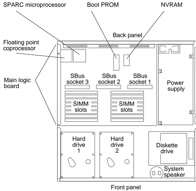
Figure 1-2 Top View With the Cover Removed
