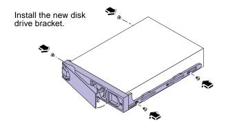
4. Repeat steps 1 to 3 as many times as is necessary to install the new disk drive brackets onto your 1-inch high disk drives.
