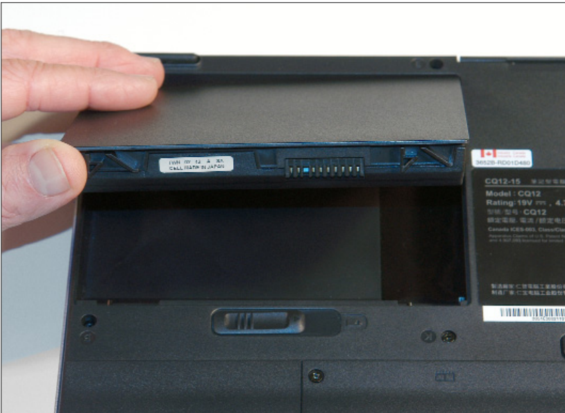
Figure 2-1: Installing the battery
