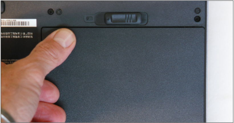
Figure 3-3: Inserting the battery
