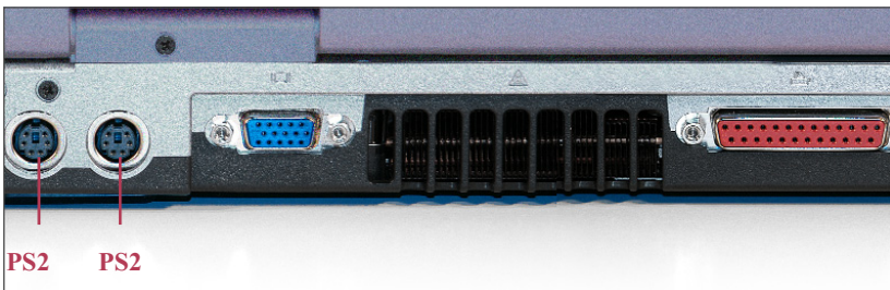
Figure 3-30: PS2 (keyboard/mouse) ports on back panel
