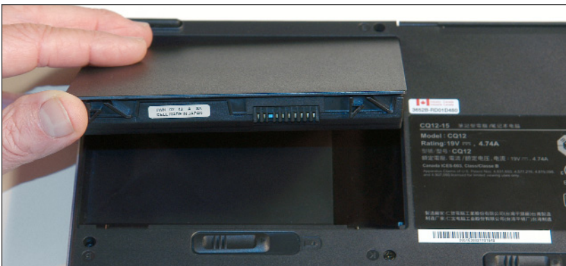
Figure 3-5: Removing the battery
