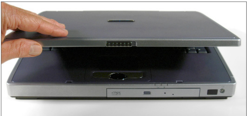
Figure 3-1: Opening the display cover
