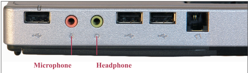
Figure 3-28: Microphone and Headphone ports
