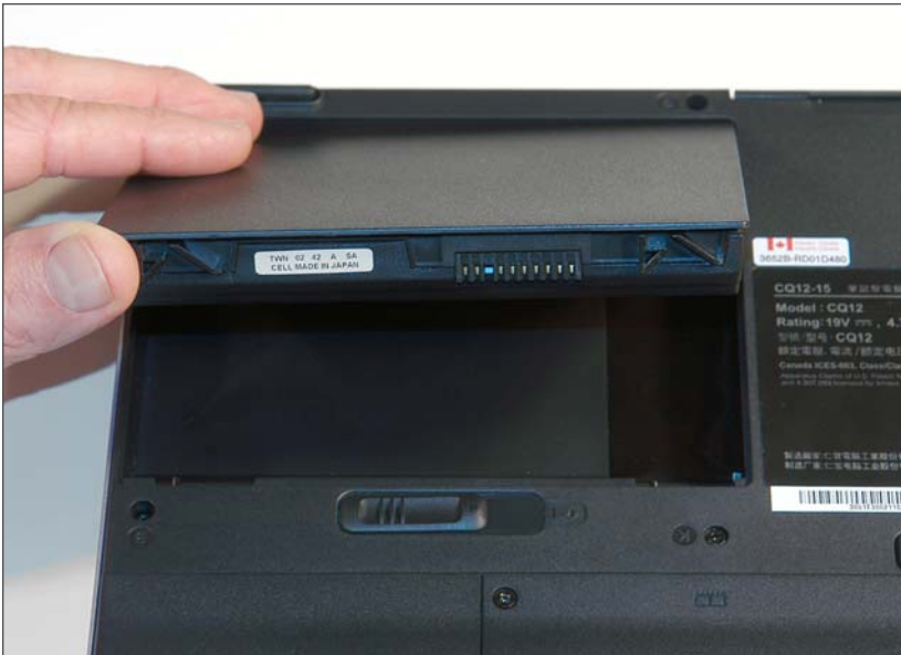
Figure 2-1: Installing the battery
