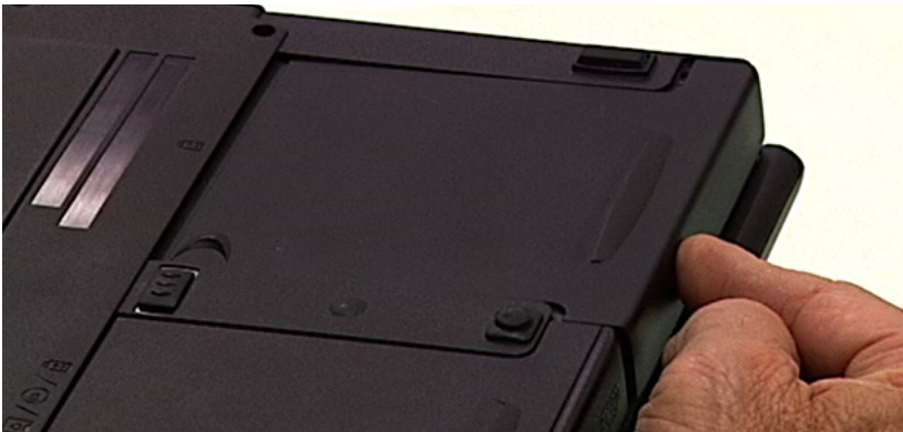
Figure 3-3: Inserting the battery pack
