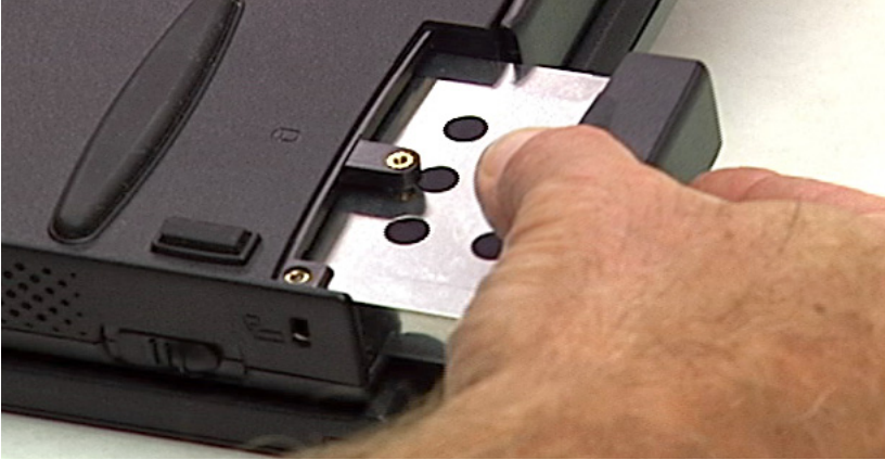
Figure 3-6: Removing the internal hard drive
