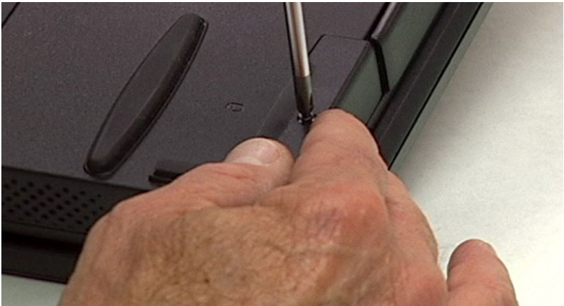
Figure 3-5: Removing the hard drive locking screw
