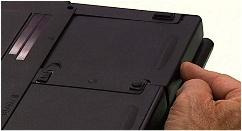
Figure 2-2: Installing the battery pack
