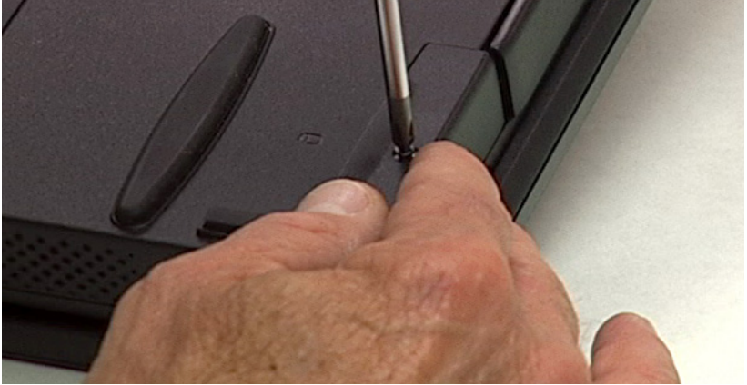
Figure 3-8: Re-installing the hard drive locking screw
