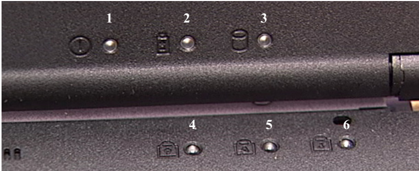
Figure 3-21: System status indicators
