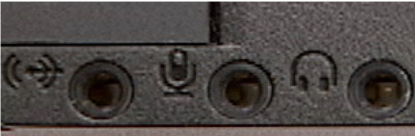
Figure 3-25: Audio ports (from left to right: Line-in, External microphone, Line-out)
