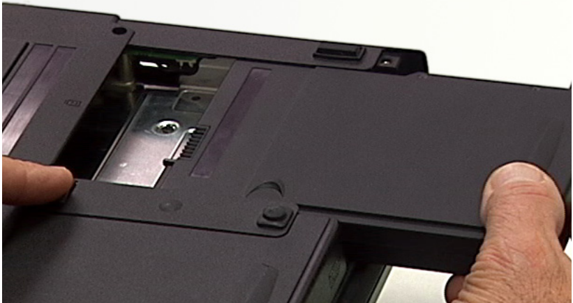
Figure 3-4: Removing the battery pack
