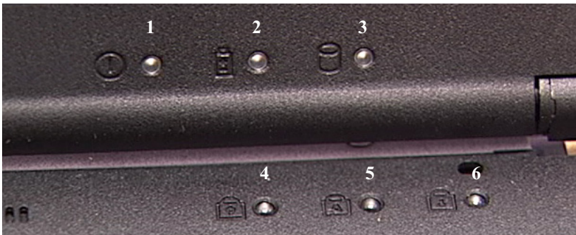
Figure 9-6: The system status indicator LEDs
