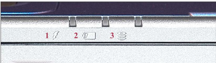
**Figure 3-31: System status LEDs on the front panel**
