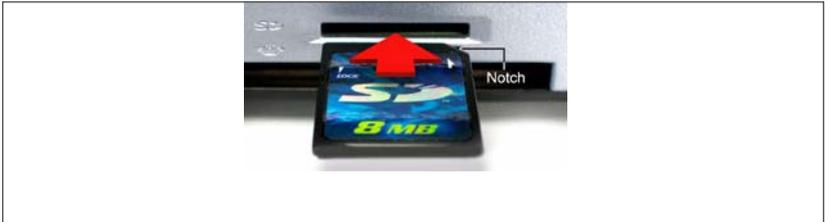
**Figure 3-16: Inserting a Secure Digital card**
