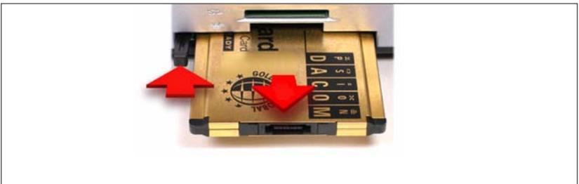
**Figure 3-10: Removing the PC card**
