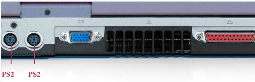
**Figure 3-30: PS2 (keyboard/mouse) ports on back panel**
