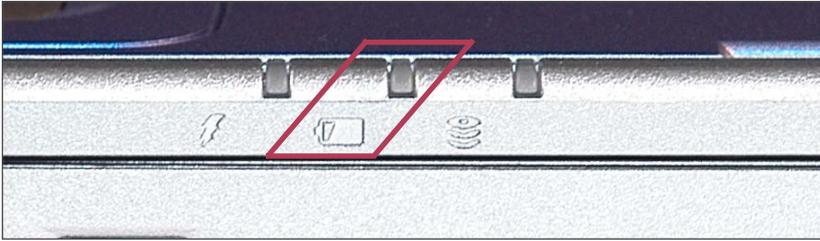
Figure 3-4 Front panel battery status LED
