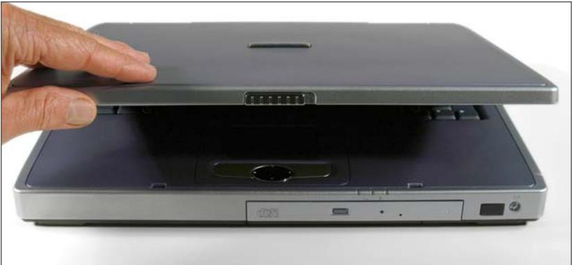
**Figure 3-1: Opening the display cover**
