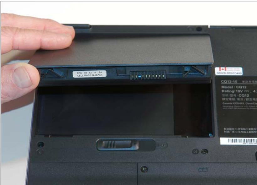
Figure 2-1: Installing the battery
