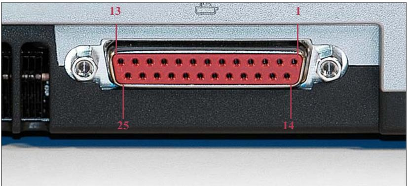
Figure A-6: Parallel port connector
