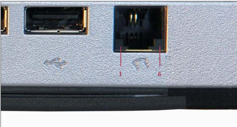
Figure A-5: Serial port connector
