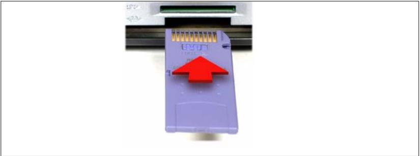
**Figure 3-12: Inserting a Memory Stick card**
