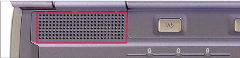
Figure 3-26: Left (channel) stereo speaker
