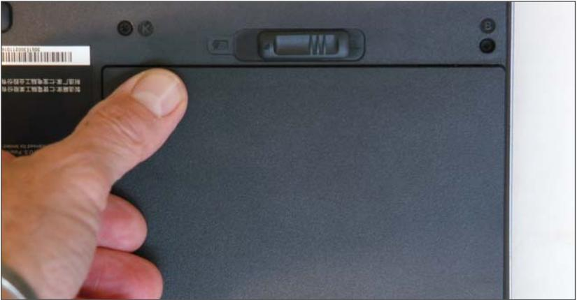
Figure 3-3: Inserting the battery
