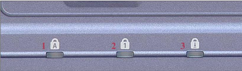
Figure 3-32: System status LEDs above the keyboard
