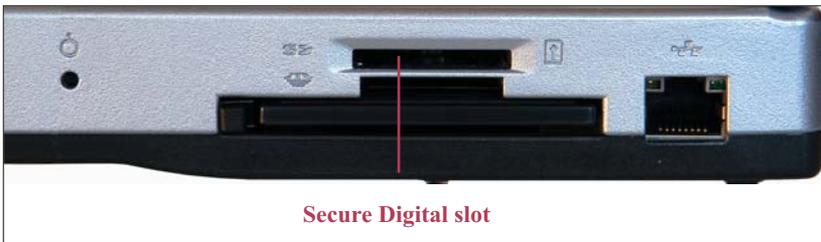
Figure 3-15: Secure Digital slot
