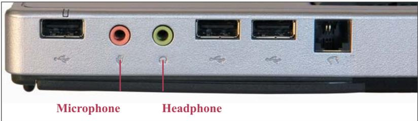
**Figure 3-28: Microphone and Headphone ports**
