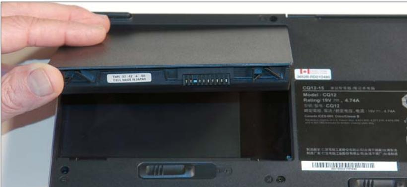
Figure 3-5: Removing the battery
