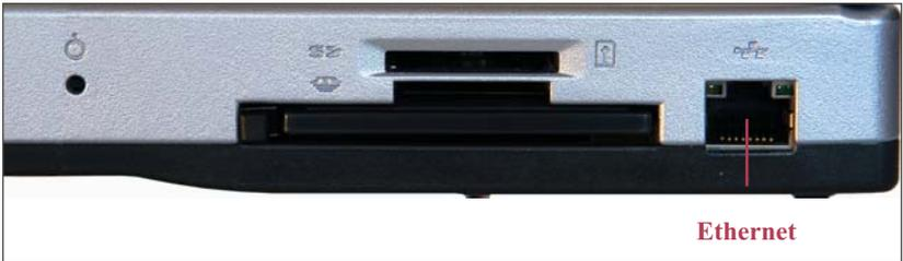
Figure 3-20: RJ-45 Ethernet port
