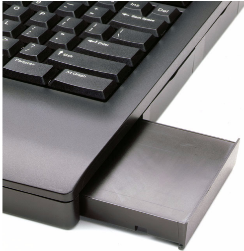
Figure 2-1 Battery Partially Inserted
