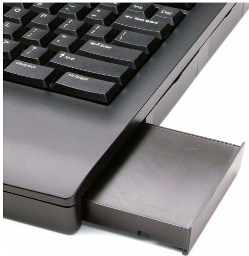
Figure 9-6 Battery and Battery Device Bay
