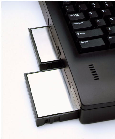
Figure 3-8 Partially Inserted Disk Drives
