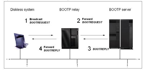
The server replies to the broadcast with either a broadcast or unicast back to the client. The BOOTP request and replies contain a vendor-specific area which allows transmission of system information like subnet mask, hostname, domain name, default gateway, name servers, and other information.
