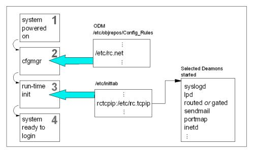
Figure 21. TCP/IP network startup procedure
