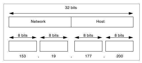
Figure 7. IP address format
