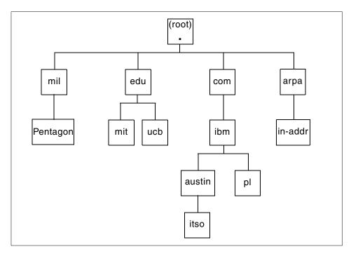
Figure 32. DNS structure
