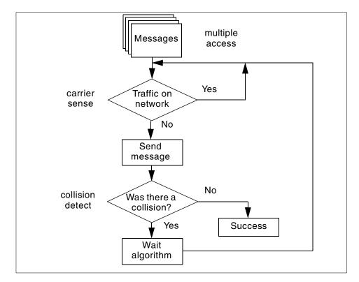
Figure 4. CSMA/CD algorithm
