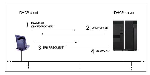
Figure 25. The DHCP client-server simple request message flow.
