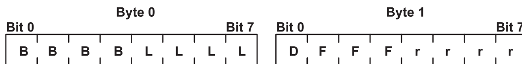
Figure 26. Routing Control Field. This illustration shows byte 0 and byte 1 of a routing control field. The eight bits of byte one are B, B, B, B, L, L, L, L. The eight bits of byte 1 are D, F, F, F, r, r, r, r.
