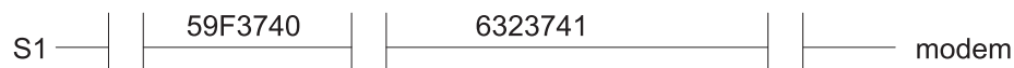
Figure 35. Modem to Native Serial Port Cable Assembly. This illustration shows a 59F3740 cable on the serial port end and a 6323741 on the modem end.
