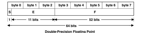
Figure 13. Double-Precision Floating-Point. The first line of this diagram lists bytes 0 through 7. The second line of the diagram shows the corresponding fields and their respective lengths: S (1 bit) and E (11 bits) extend under byte 0 through byte 2, while F (52 bits) extends from byte 3 to byte 7. The third line shows the total length of bytes 0 through 7, which is 64 bits.
