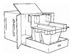
4 Remove the packing foam from the UNIX PC main unit.
