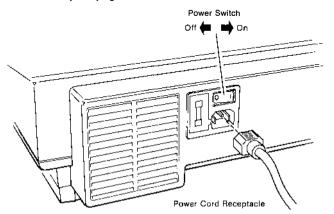
3 Plug the black power cord firmly into its receptacle located in the back of the workstation.
