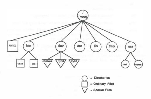
Figure 1-4. Example of a File System
