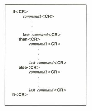
Figure 7-5. Format of the if...then...else Conditional Construct
