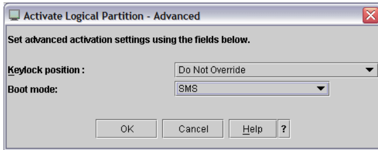
Figure 3-33 Partition activation - Advanced, selection of SMS
