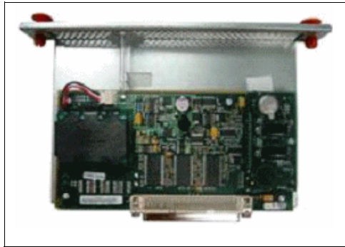
Figure 2-9 Raid5 adapter with write cache
