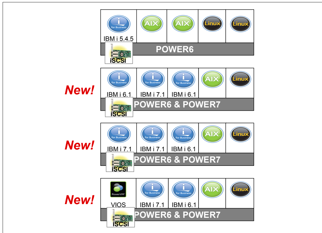
Figure 8-11 Additional OS levels combinations of server and client for IBM i and VIOS
