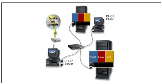
Figure 3-10 HMC with indirect network attach
