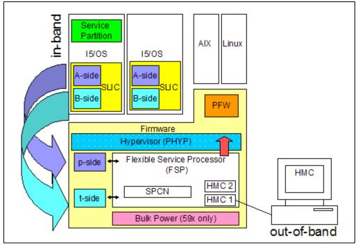
Figure 14-26 shows an overview of the firmware update process.
