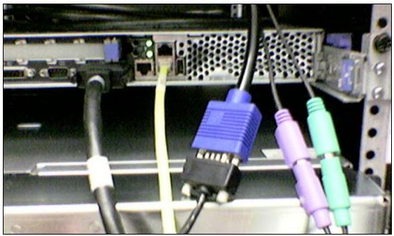
Figure 3-6 Rear view of rack mounted HMC ports
