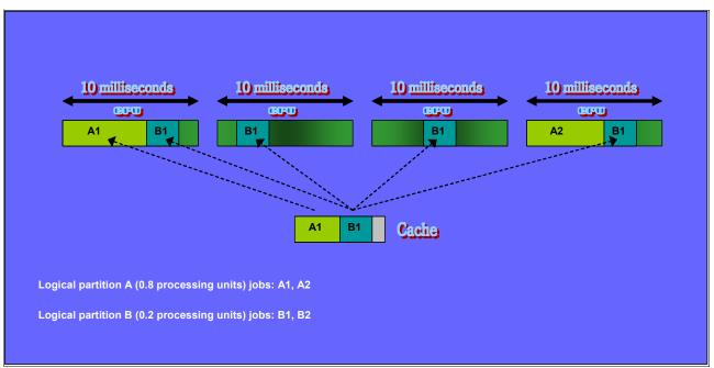
Figure 1-7 Two logical partitions sharing one processing unit
