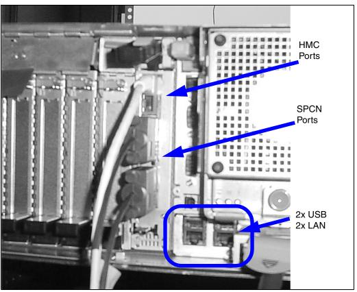
Figure 3-8 Ports on rear of i570
