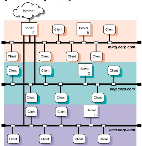
Figure 7-2: Sample Large DNS Configuration
