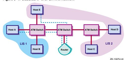
Figure 3-1: Classical IP over an ATM Network
