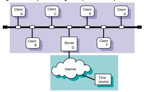
Figure 11-2: Sample NTP Configuration (Internet Source)
