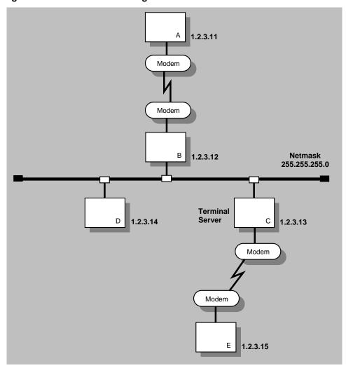
Figure 5-5: Network PPP Configuration
