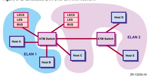
Figure 3-2: Emulated LAN over an ATM Network
