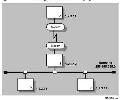
Figure 5–2: SLIP Configuration with Gateway System
