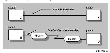
Figure 5–5 shows two PPP connections. The first is between host A and host B, with host B acting as a gateway system. The second is between personal
