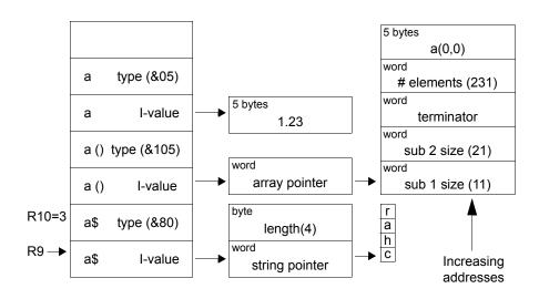
The diagram above shows the resulting parameter block and other data items when code is called. The access method into the arrays is given by the following algorithm:
