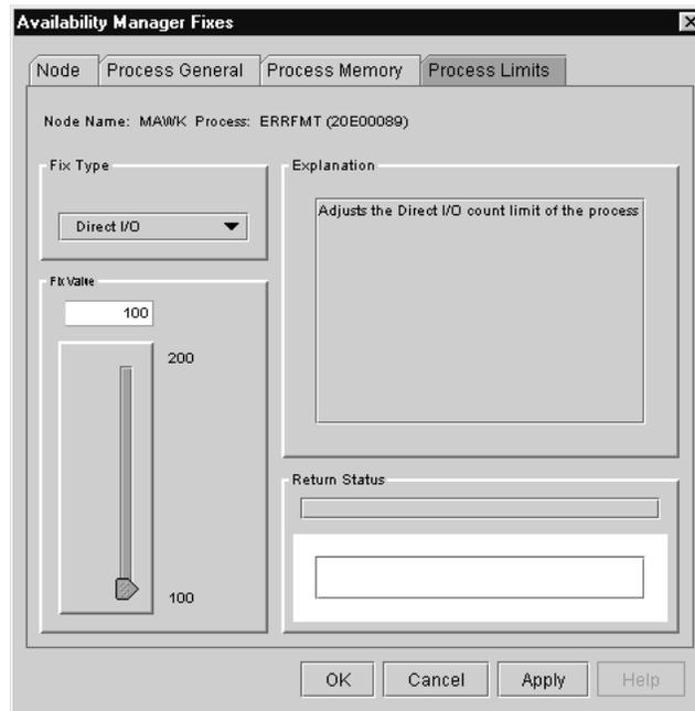
To perform this fix, use the slider to adjust the direct I/O count to the limit you want. You can also click the line above or below the slider to adjust the number by 1.
