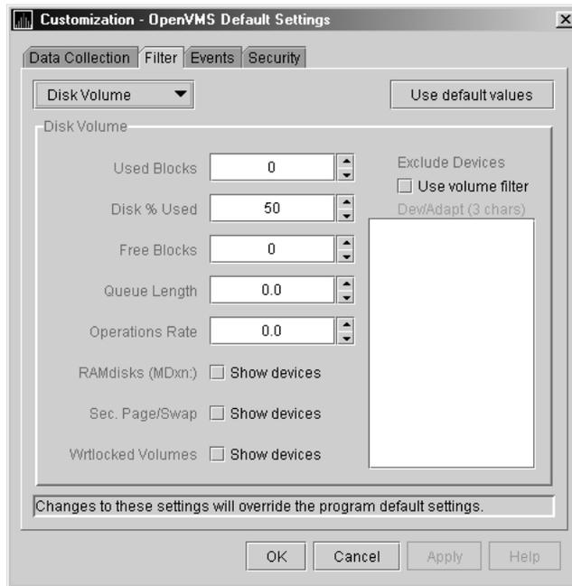
The OpenVMS Disk Volume Filters page allows you to change the values for the following data:
