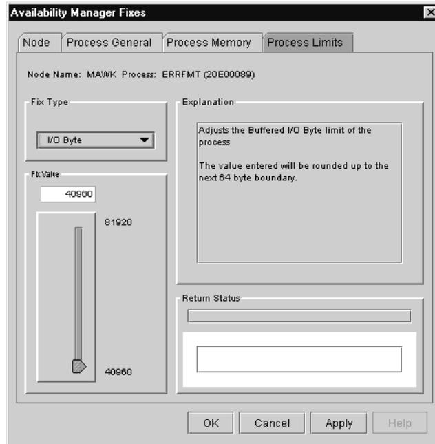
To perform this fix, use the slider to adjust the I/O byte limit to the number you want. You can also click the line above or below the slider to adjust the number by 1.
