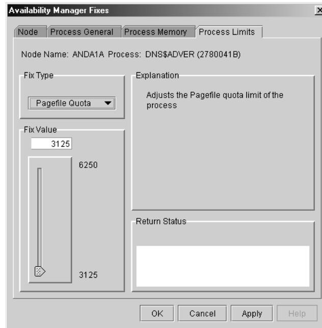
To perform this fix, use the slider to adjust the pagefile quota limit to the number you want. You can also click above or below the slider to adjust the fix value by 1.
