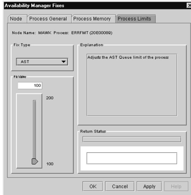
To perform this fix, use the slider to adjust the AST queue limit to the number you want. You can also click the line above or below the slider to adjust the number by 1.
