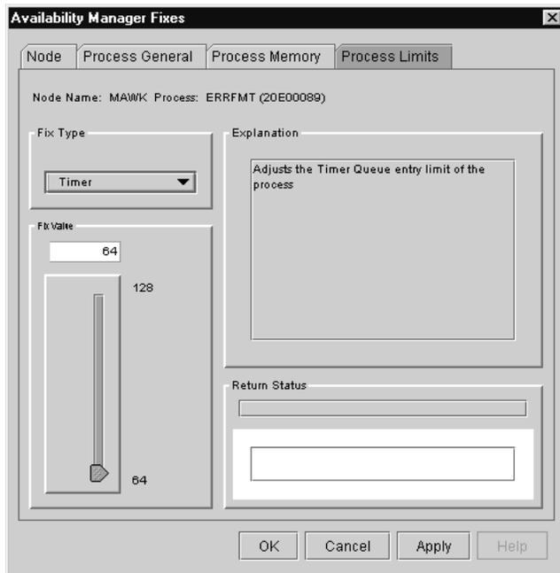
To perform this fix, use the slider to adjust the timer queue entry limit to the number you want. You can also click the line above or below the slider to adjust the number by 1.
