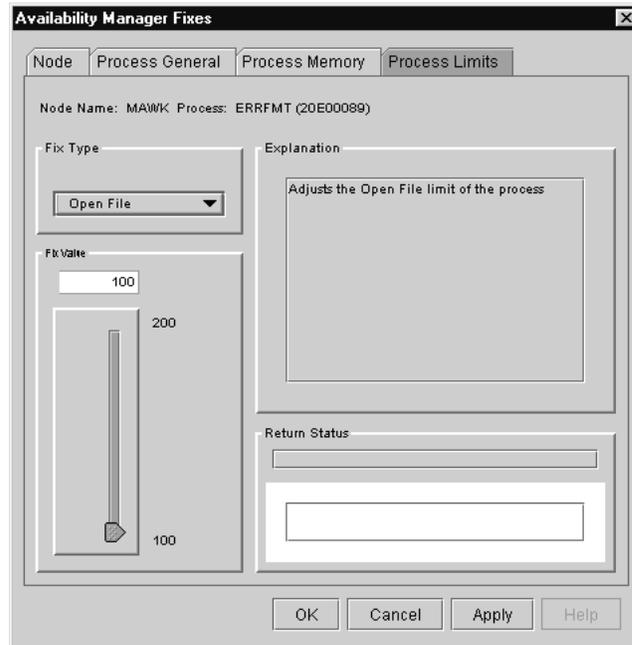
To perform this fix, use the slider to adjust the open file limit to the number you want. You can also click the line above or below the slider to adjust the number by 1.
