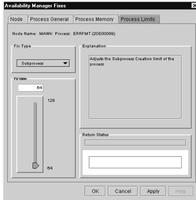
To perform this fix, use the slider to adjust the subprocess creation limit of a process to the number you want. You can also click the line above or below the slider to adjust the number by 1.
