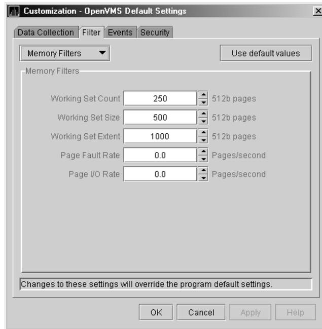
The OpenVMS Memory page (Figure 3–9) displays the values on this filters page. The OpenVMS Memory Filters page allows you to change values for the following data:
