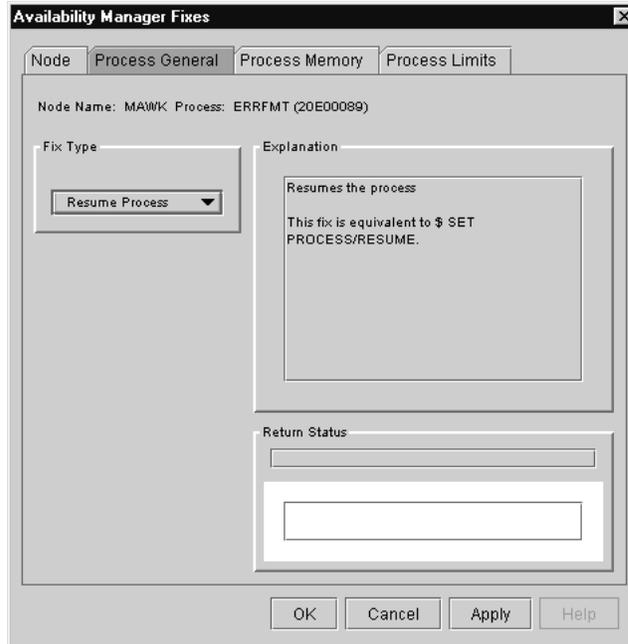
After reading the explanation, click **Apply** at the bottom of the page to apply the fix. A message displayed on the page indicates that the fix has been successful.
