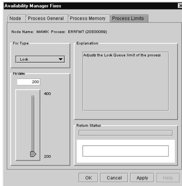
To perform this fix, use the slider to adjust the lock queue limit to the number you want. You can also click the line above or below the slider to adjust the number by 1.
