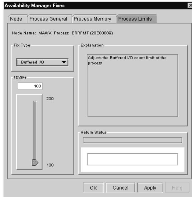
To perform this fix, use the slider to adjust the buffered I/O count to the limit you want. You can also click the line above or below the slider to adjust the number by 1.
