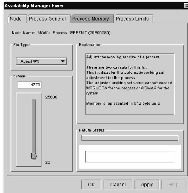
To perform this fix, use the slider to adjust the working set to the limit you want. You can also click the line above or below the slider to adjust the number by 1.
