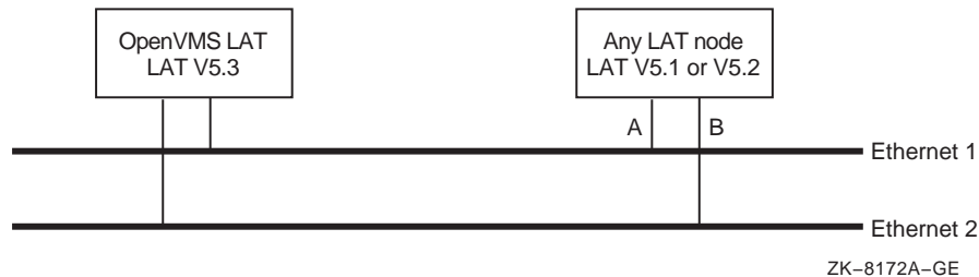
Figure 24–5 Unsupported Multiple Address LAT Configuration
