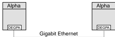
Figure 3–2 Point-to-Point Gigabit Ethernet OpenVMS Cluster Configuration
